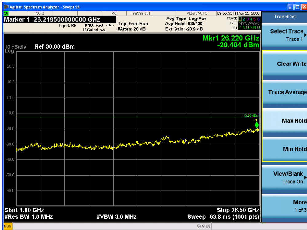
Conducted Spurious Emissions Downlink Low CH (1 GHz – 26.5 GHz-Cellular)
