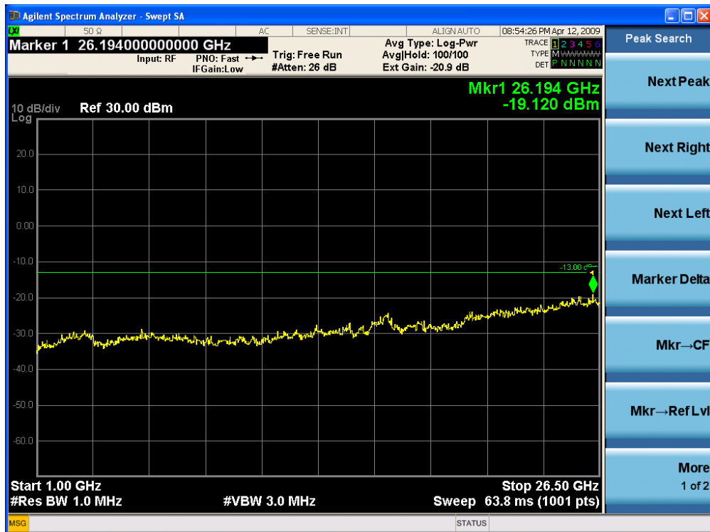
Conducted Spurious Emissions Uplink Low CH (1 GHz – 26.5 GHz-Cellular)
