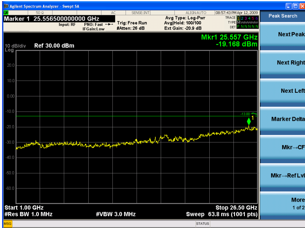
Conducted Spurious Emissions Downlink High CH (1 GHz – 26.5 GHz-Cellular)
