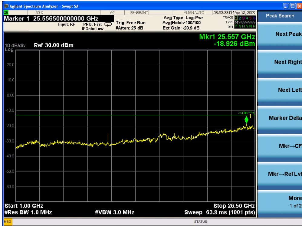
Conducted Spurious Emissions Uplink Mid CH (1 GHz – 26.5 GHz-Cellular)
