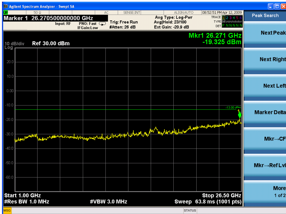
Conducted Spurious Emissions Uplink High CH (1 GHz – 26.5 GHz-Cellular)
