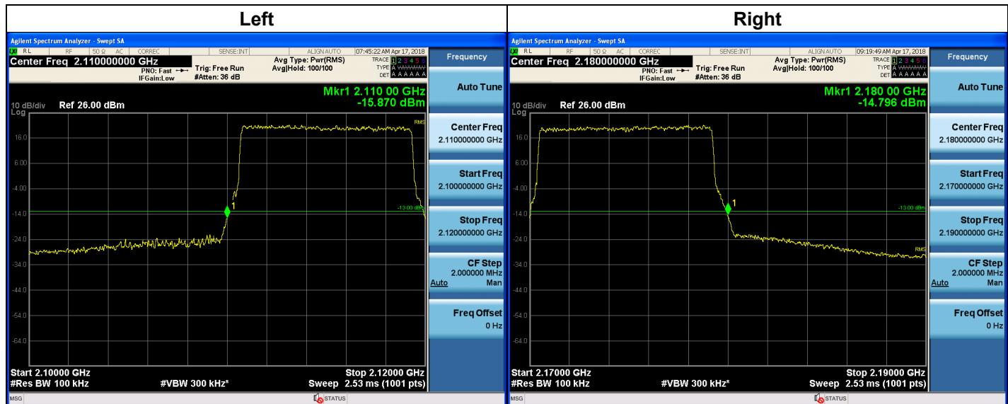
**Plot of Intermodulation for LTE 10 MHz**
