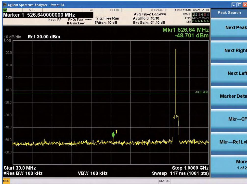
**Conducted Spurious Emissions Uplink HighCH (30 MHz – 1 GHz-Cellular)**
