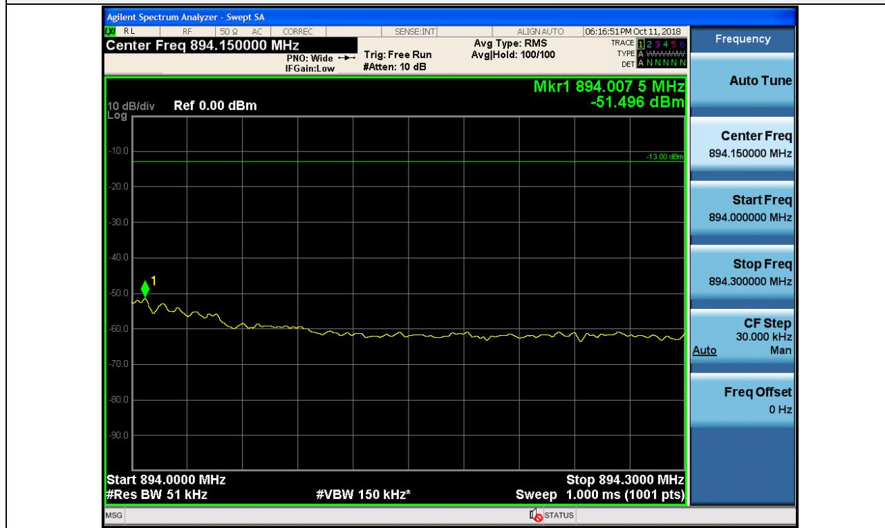
+3 dB above Out-of-band (two adjacent test signals) / Cellular / Downlink / LTE 5 MHz / Lower
