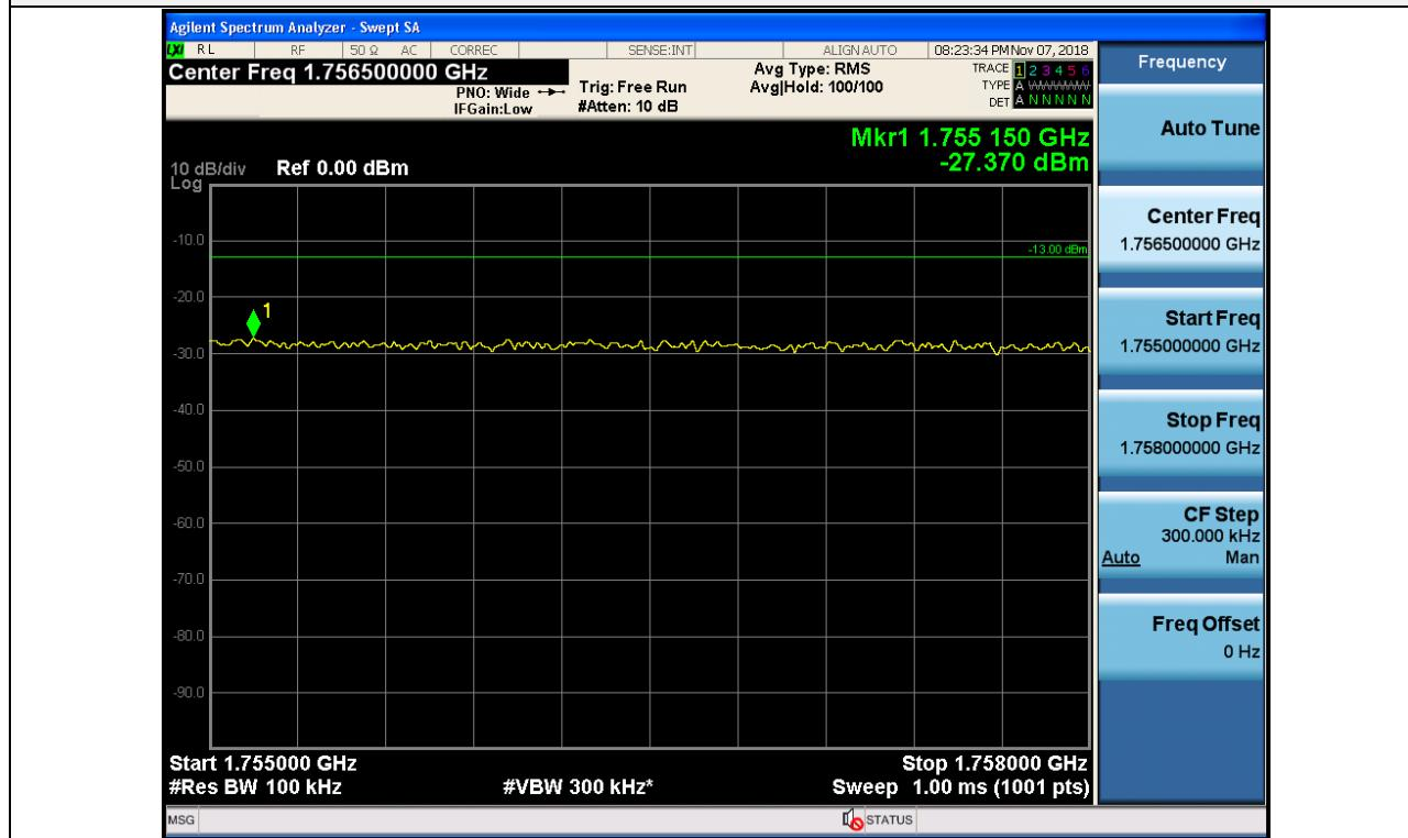
+3 dB above Out-of-band (two adjacent test signals) / AWS-1 / Uplink / LTE 10 MHz / Lower
