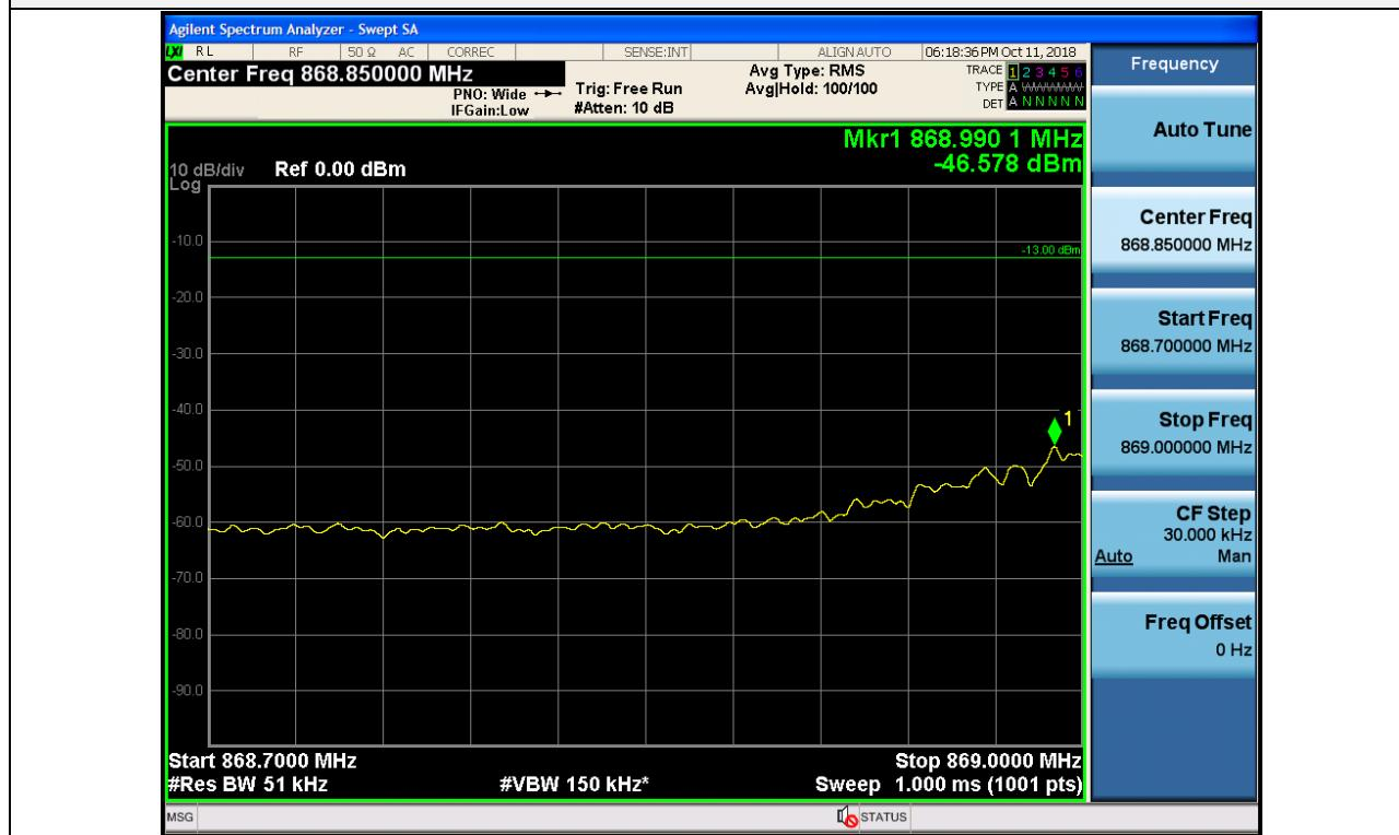
+3 dB above Out-of-band (single test signal) / AWS-1 / Uplink / LTE 10 MHz / Upper
