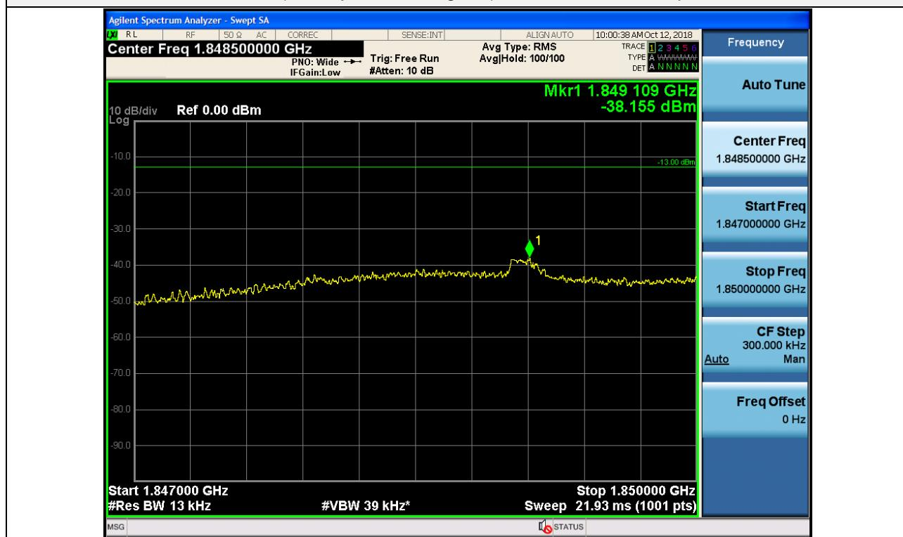
+3 dB above Out-of-band (two adjacent test signals) / Broadband PCS / Uplink / LTE 20 MHz / Upper
