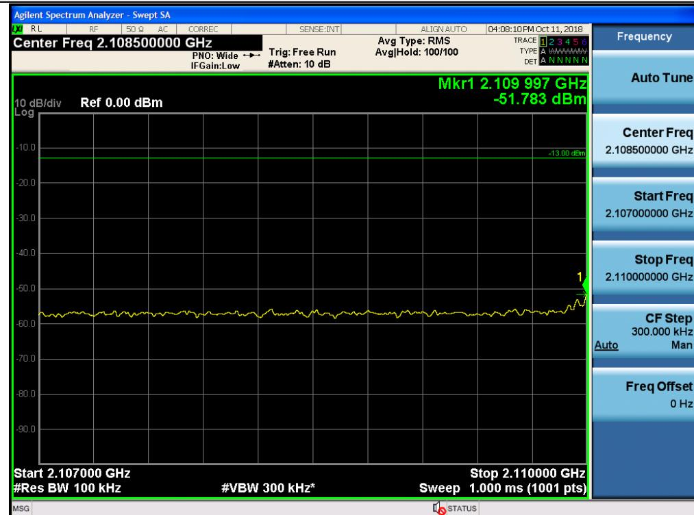
+3 dB above Out-of-band (two adjacent test signals) / Broadband PCS / Uplink / CDMA / Upper
