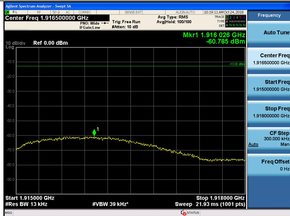
Out-of-band (two adjacent test signals) / Broadband PCS / Uplink / CDMA / Lower
