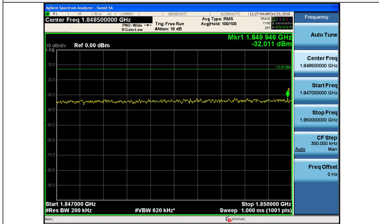
+3 dB above Out-of-band (two adjacent test signals) / Broadband PCS / Downlink / CDMA / Upper
