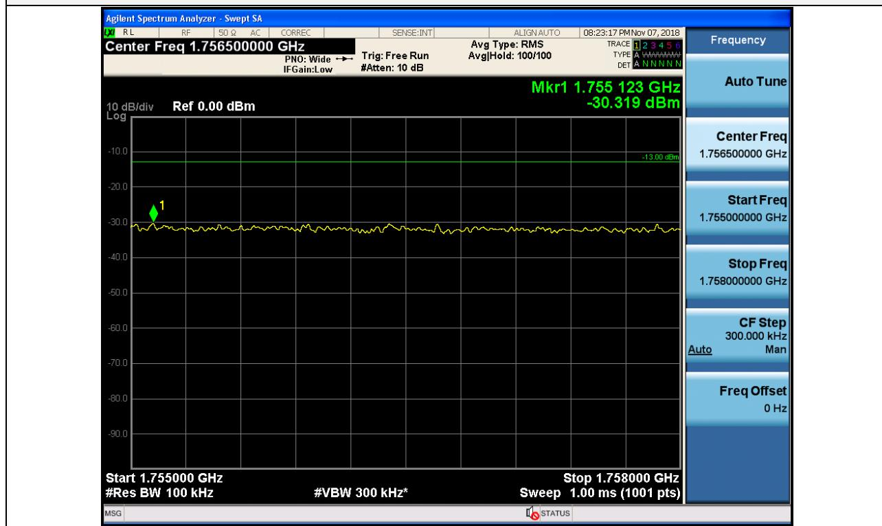
Out-of-band (two adjacent test signals) / AWS-1 / Uplink / LTE 10 MHz / Lower
