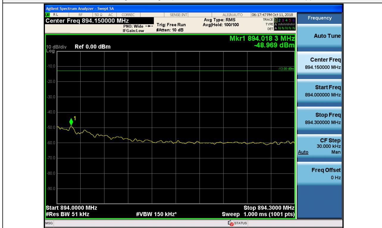
Out-of-band (single test signal) / Cellular / Downlink / LTE 5 MHz / Lower
