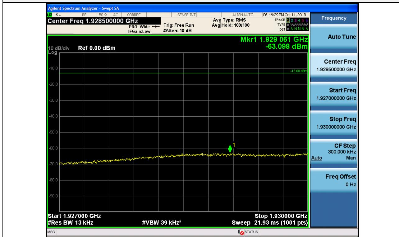
+3 dB above Out-of-band (two adjacent test signals) / Broadband PCS / Downlink / LTE 20 MHz / Upper
