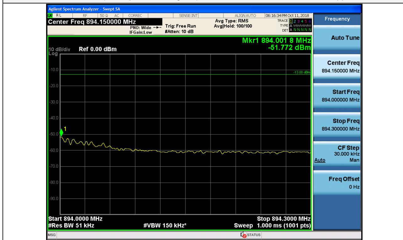
Out-of-band (two adjacent test signals) / Cellular / Downlink / LTE 5 MHz / Lower
