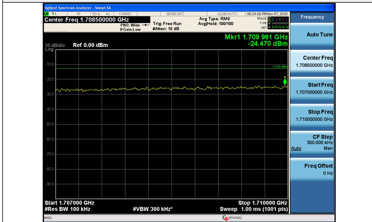
+3 dB above Out-of-band (two adjacent test signals) / AWS-1 / Downlink / LTE 10 MHz / Upper
