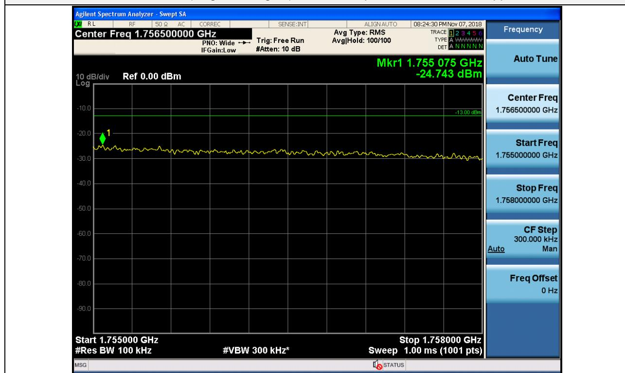
Out-of-band (single test signal) / AWS-1 / Uplink / LTE 10 MHz / Lower
