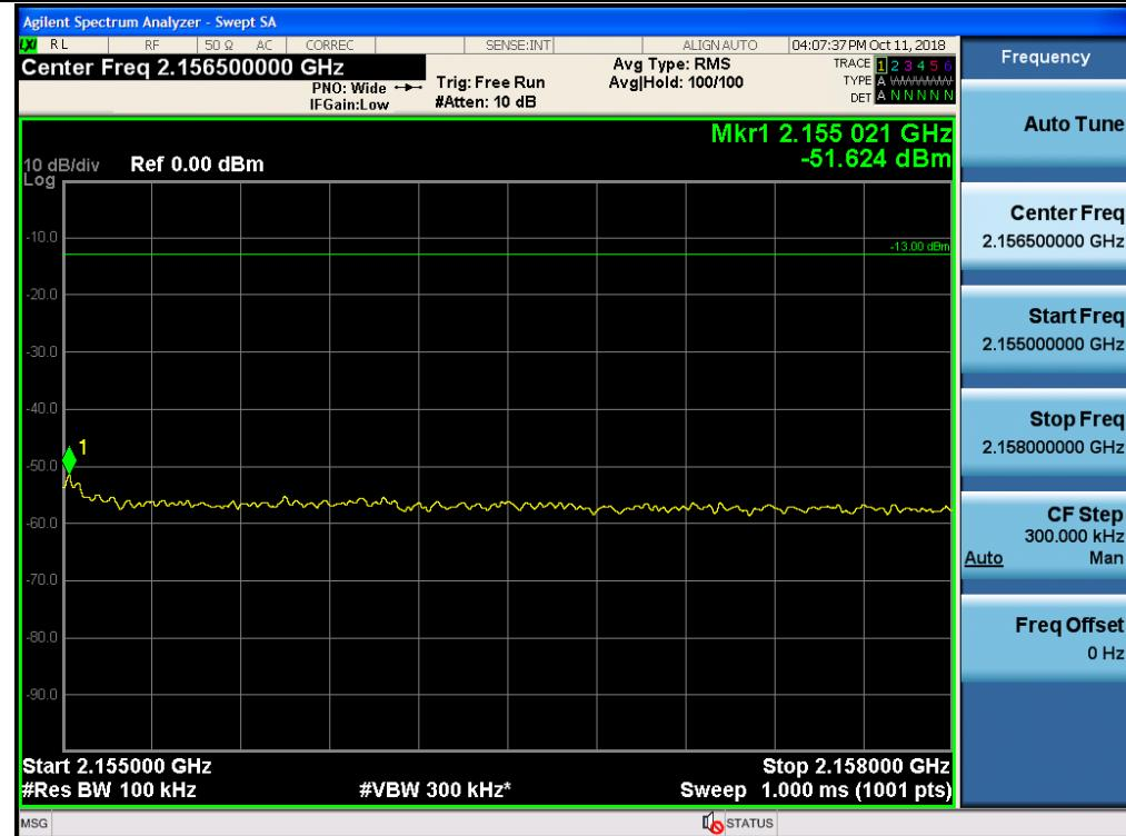
+3 dB above Out-of-band (two adjacent test signals) / AWS-1 / Downlink / LTE 10 MHz / Lower
