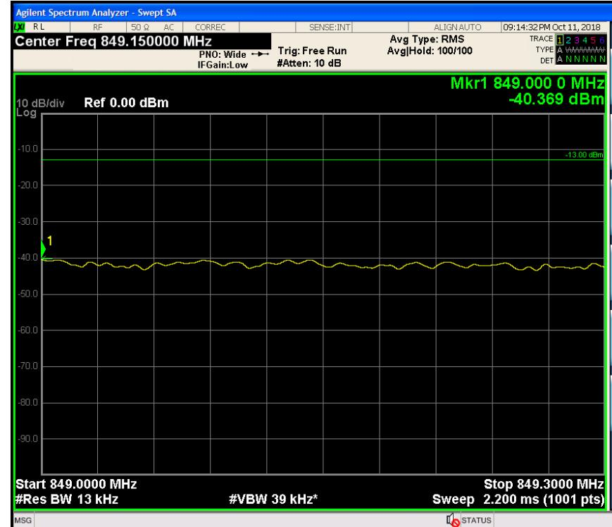
+3 dB above Out-of-band (two adjacent test signals) / Cellular / Uplink / CDMA / Lower
