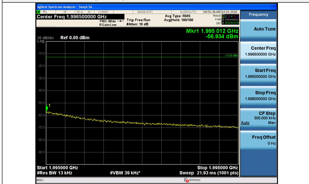
Out-of-band (single test signal) / Broadband PCS / Downlink / CDMA / Lower
