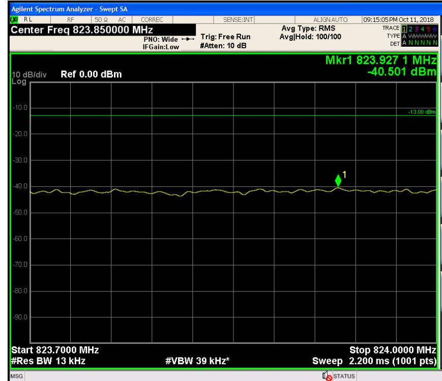
+3 dB above Out-of-band (two adjacent test signals) / Cellular / Uplink / LTE 5 MHz / Upper
