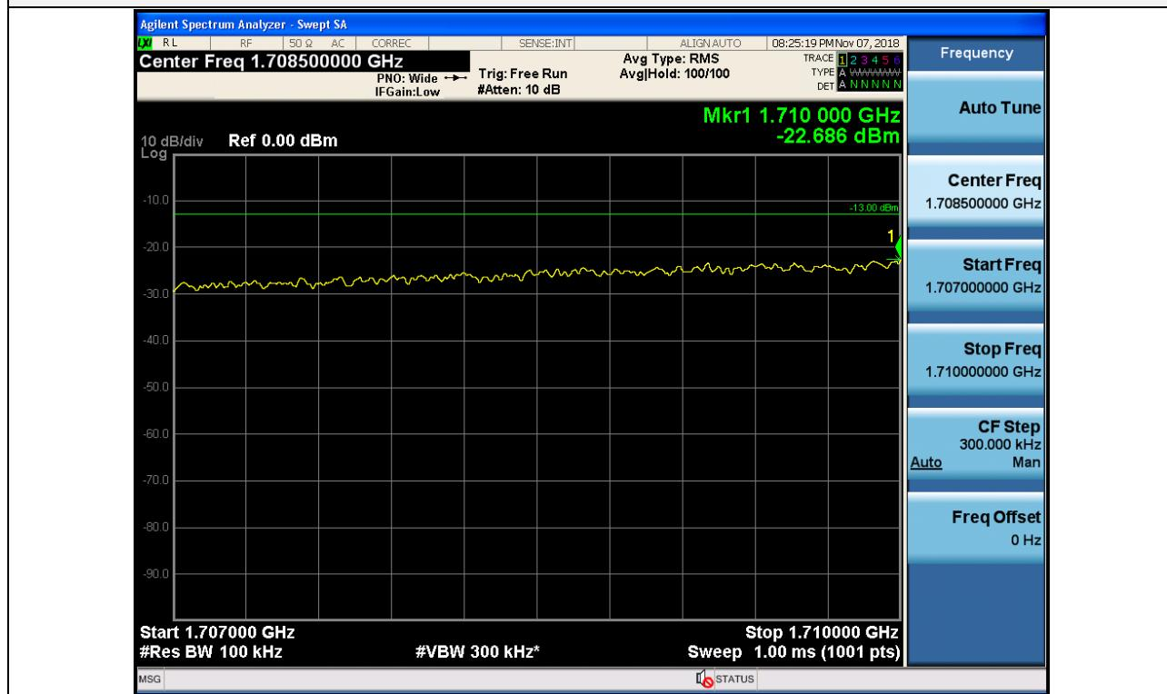
+3 dB above Out-of-band (single test signal) / AWS-1 / Downlink / LTE 10 MHz / Upper
