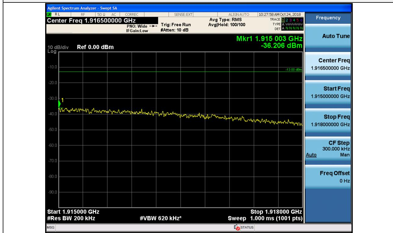
+3 dB above Out-of-band (two adjacent test signals) / Broadband PCS / Uplink / LTE 20 MHz / Lower
