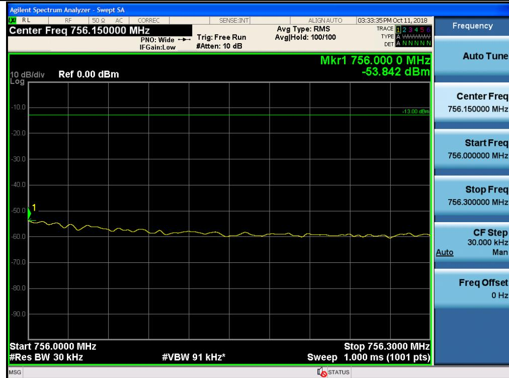
+3 dB above Out-of-band (single test signal) / Upper 700 MHz / Downlink / LTE 10 MHz / Lower
