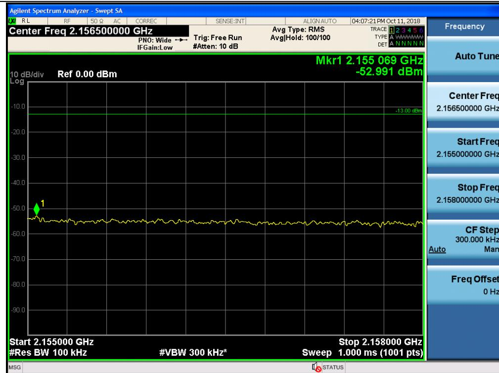
Out-of-band (two adjacent test signals) / AWS-1 / Downlink / LTE 10 MHz / Lower
