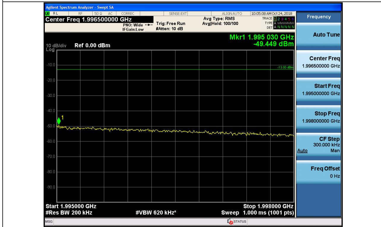
+3 dB above Out-of-band (single test signal) / Broadband PCS / Downlink / LTE 20 MHz / Lower
