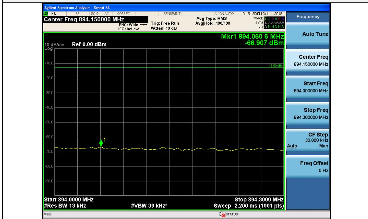
+3 dB above Out-of-band (two adjacent test signals) / Cellular / Downlink / CDMA / Lower
