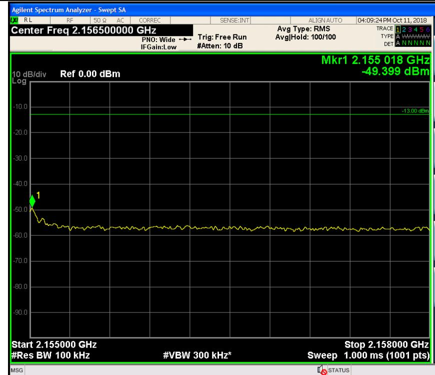
+3 dB above Out-of-band (single test signal) / AWS-1 / Downlink / LTE 10 MHz / Lower
