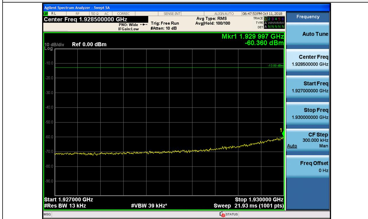
+3 dB above Out-of-band (single test signal) / Broadband PCS / Downlink / LTE 20 MHz / Upper
