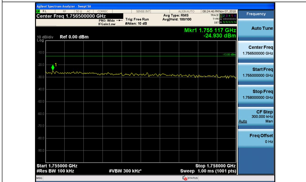
+3 dB above Out-of-band (single test signal) / AWS-1 / Uplink / LTE 10 MHz / Lower
