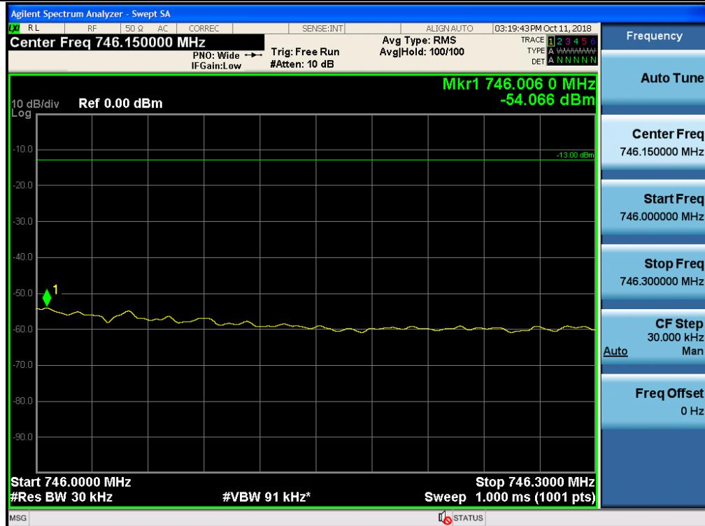
Out-of-band (single test signal) / Lower 700 MHz / Downlink / LTE 10 MHz / Lower
