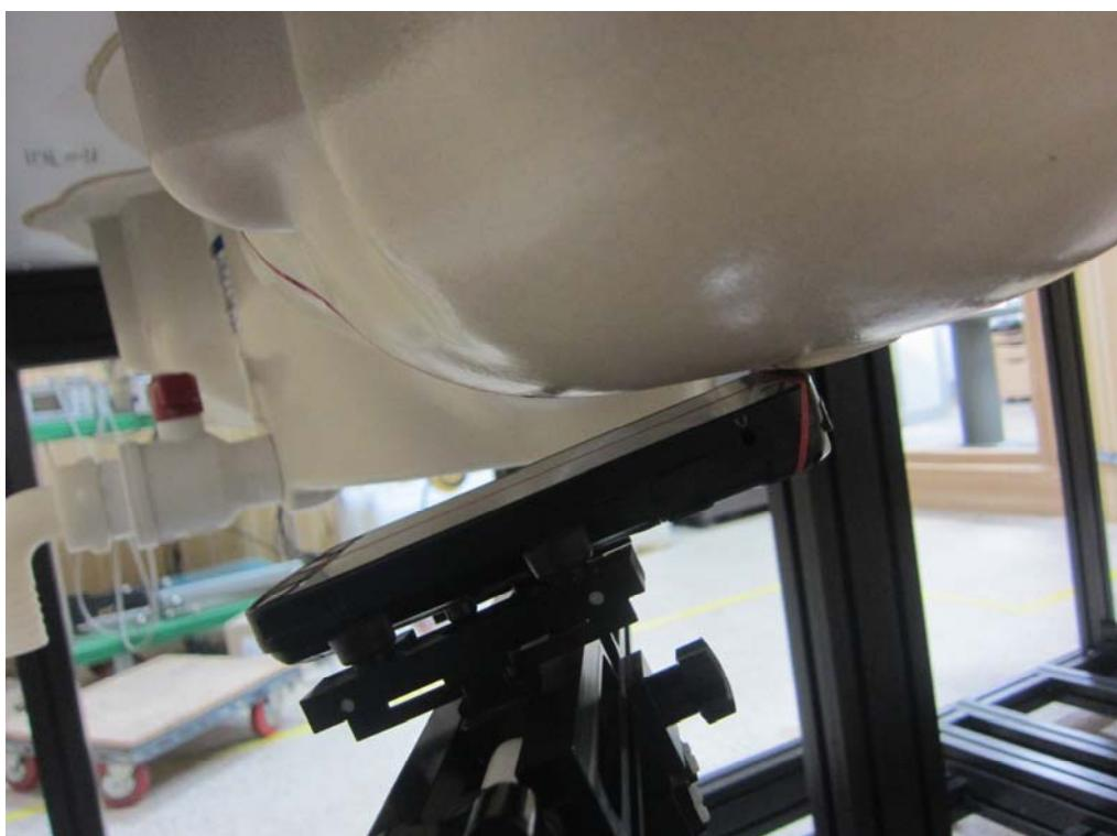
**■ Test Setup Photo (Body-Worn SAR Test Photo)**
