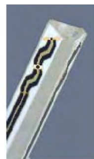
Figure E.2.2 Probe Thick-Film Technique
