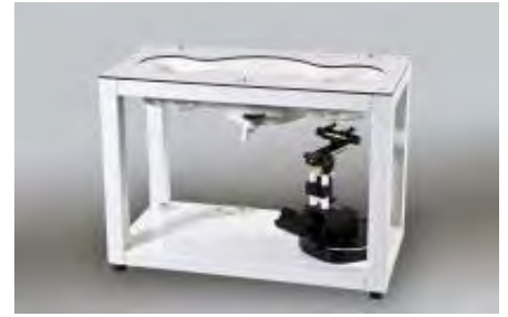
Figure E.5.1 SAM Twin Phantom
