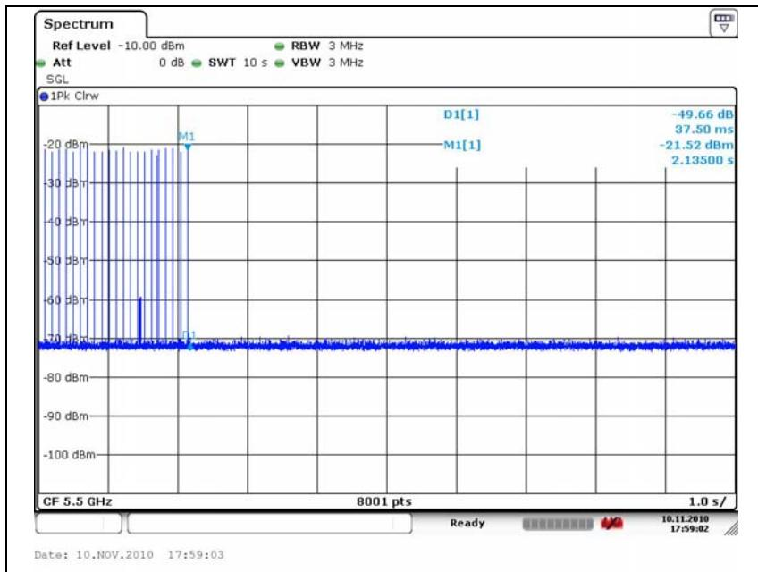
**Plot of aggregate channel closing transmission time**
