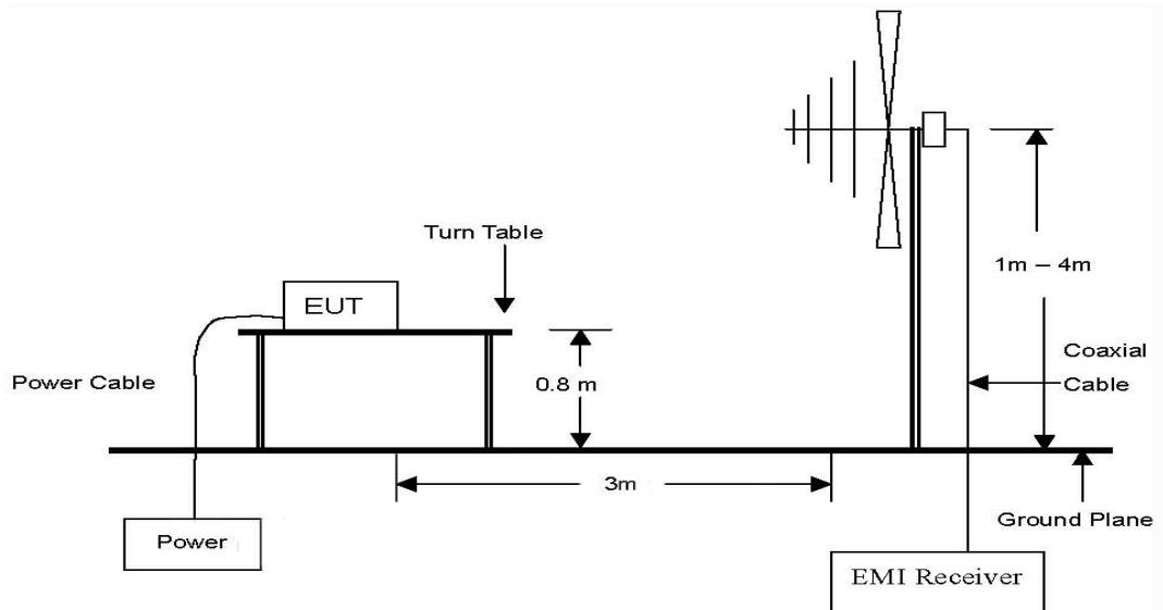
The diagram below shows the test setup that is utilized to make the measurements for emission from 1 GHz to 40 GHz Emissions.
