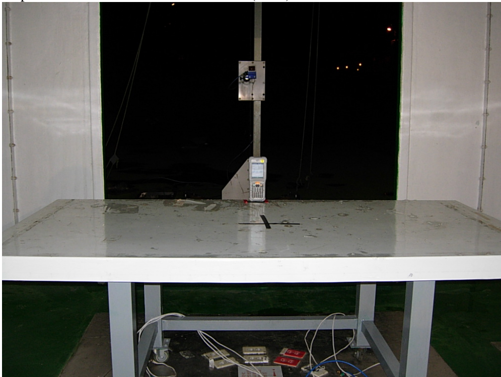
Description : Front View of Radiated Test (Horn)
