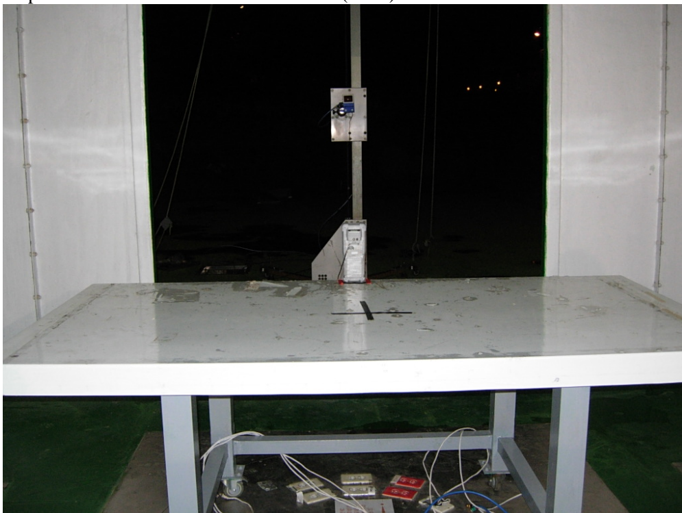
Description : Front View of Radiated Test (Horn)
