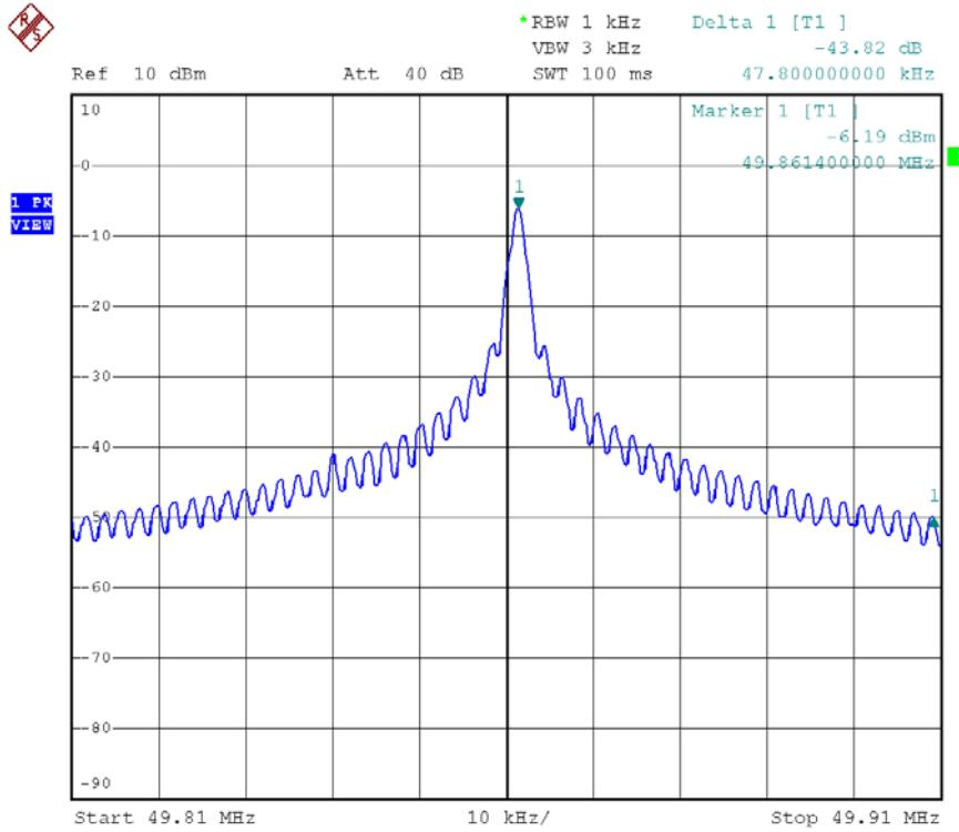
Bandwidth /Bandedge Plot – Pursuant to FCC Part 15 Section 15. 235 Requirement (Pass/Fail)
