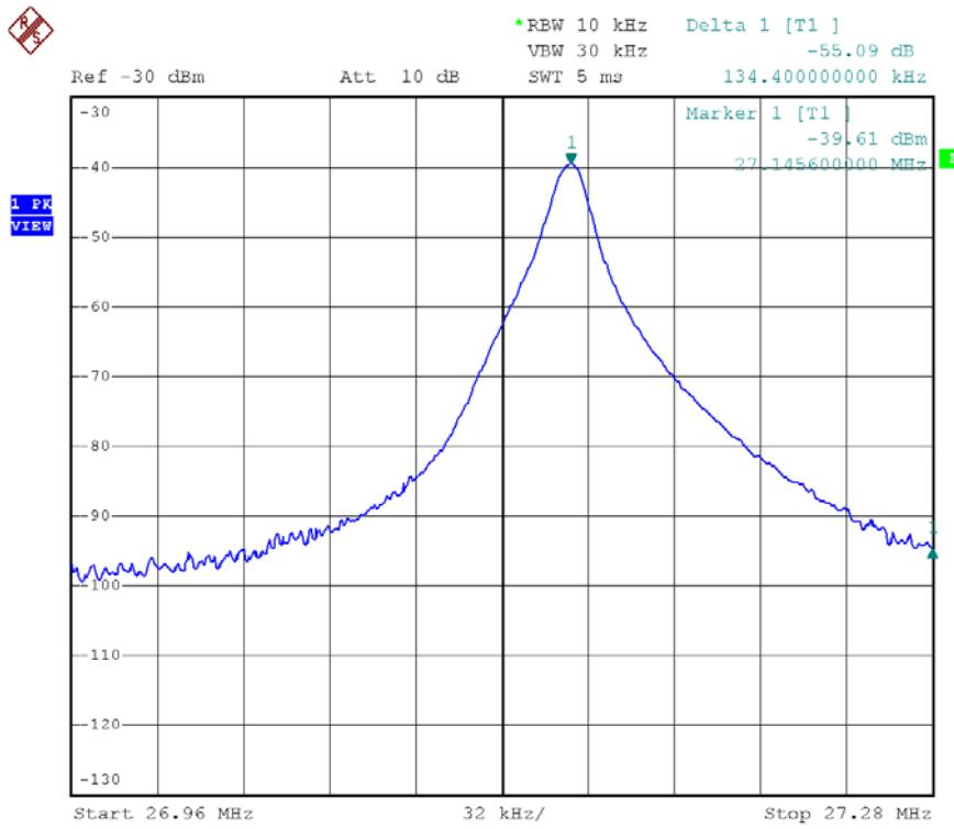
Bandwidth /Bandedge Plot – Pursuant to FCC Part 15 Section 15. 227 Requirement      (Pass/Fail)
