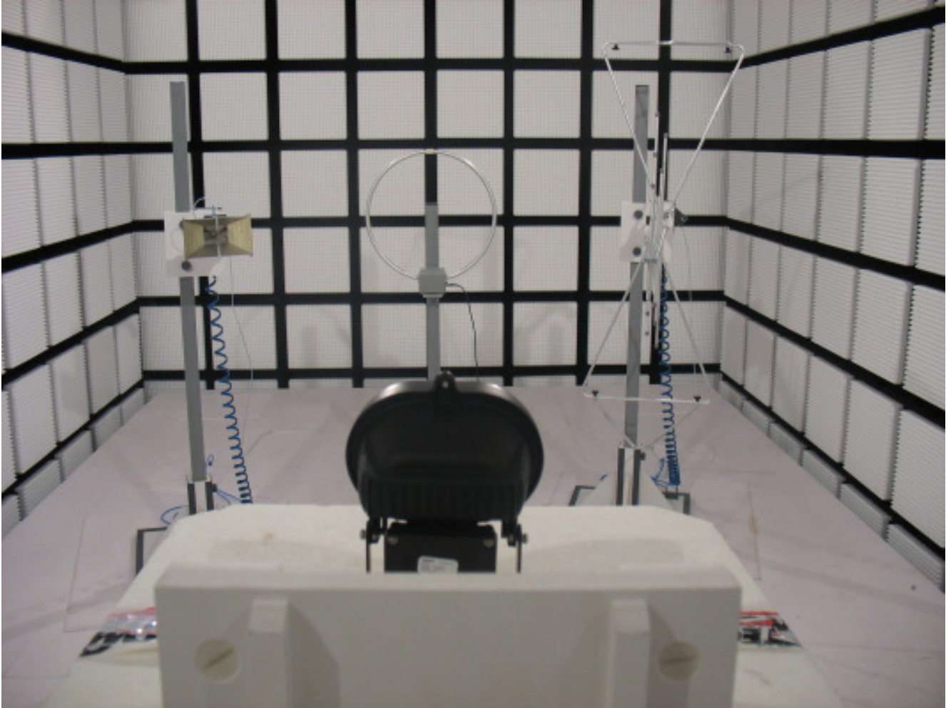
Spurious emission measurement 1 GHz – 12 GHz
