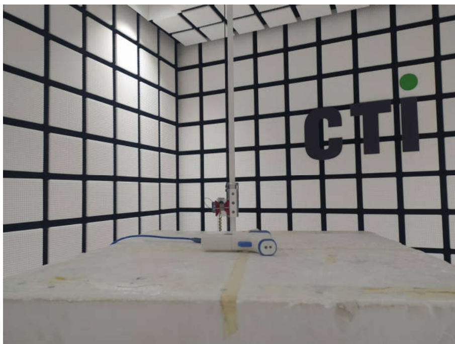
Radiated spurious emission Test Setup-2(Above 1GHz)
