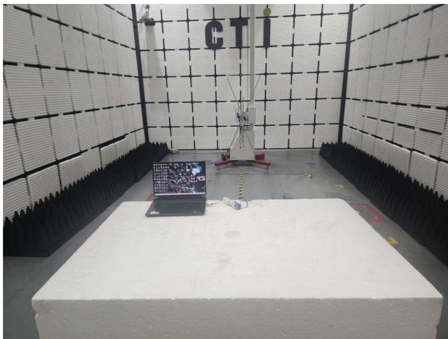
Radiated spurious emission Test Setup-1(Below 1GHz)
