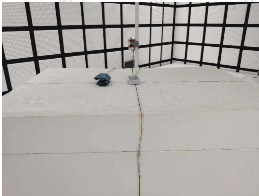
Radiated spurious emission Test Setup-3(Above 1GHz)
