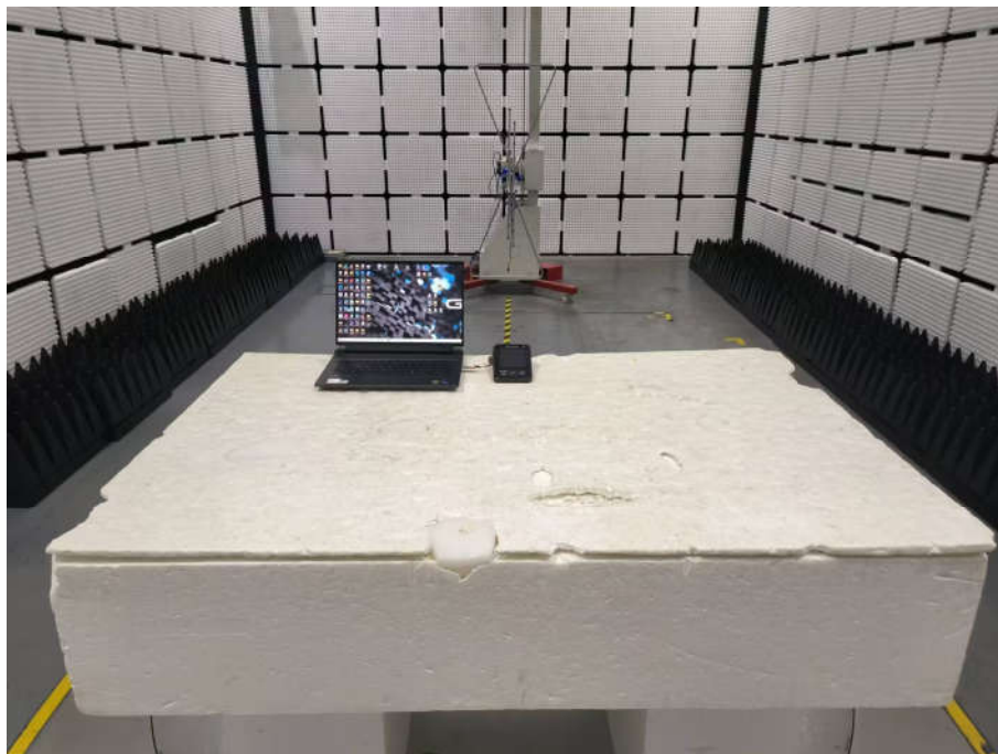
Radiated spurious emission Test Setup-1(Below 1GHz)
