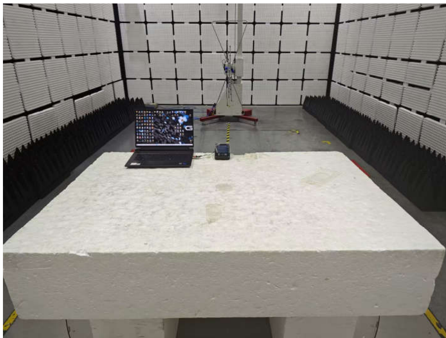
Radiated spurious emission Test Setup-1(Below 1GHz)
