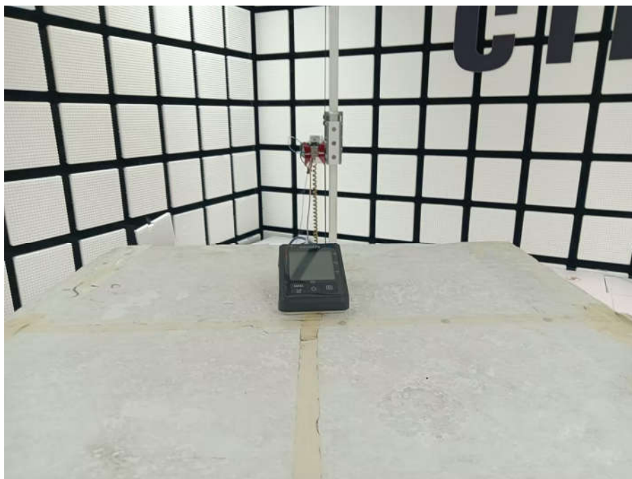
Radiated spurious emission Test Setup-2(Above 1GHz)
