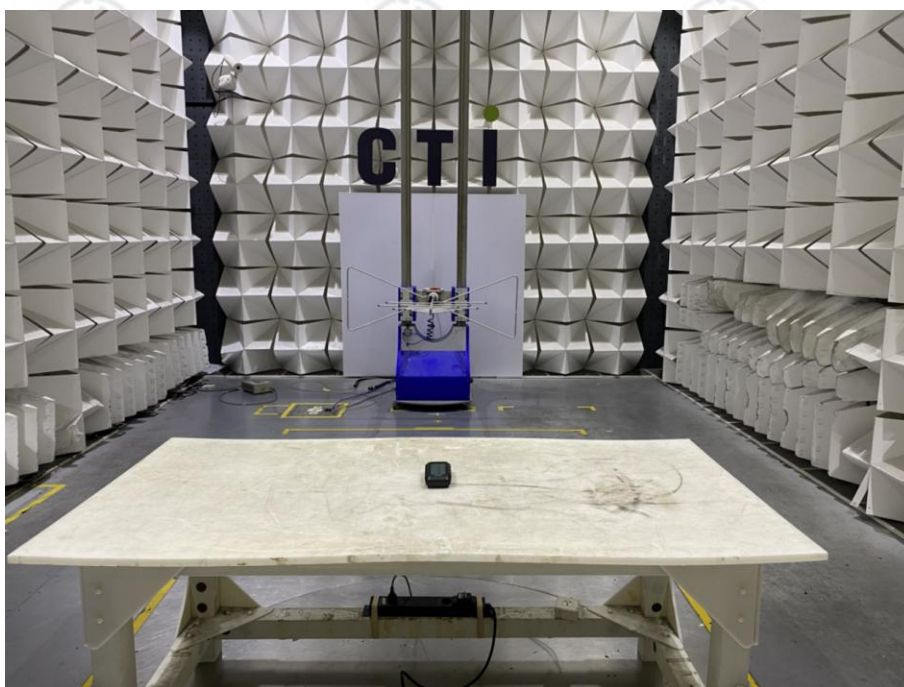
Radiated spurious emission Test Setup-1(Below 1GHz)
