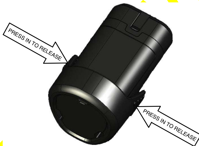
Figure 3001 HHR Battery Removal
