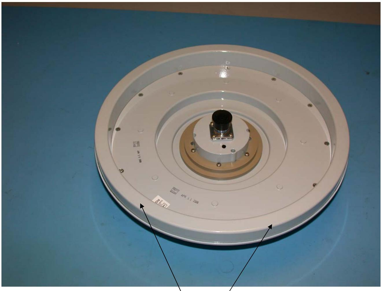
**Loop Antenna is located within the housing, approximately 10 inches in diameter**
