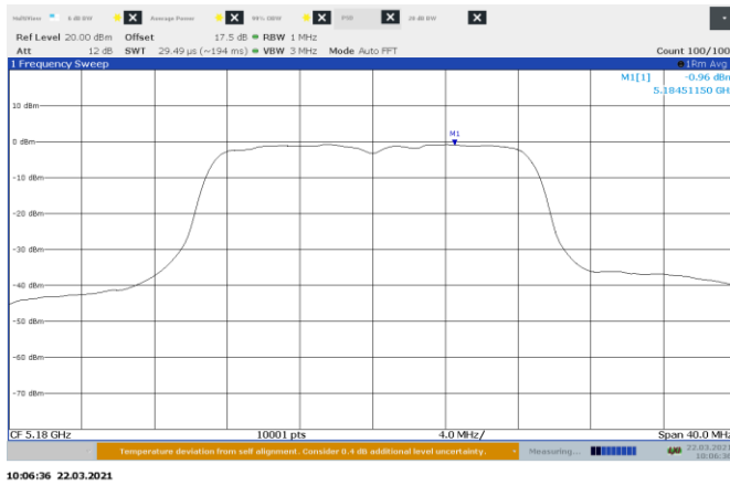
Figure 8.7-19: Conducted PSD on 802.11ac, Port A Low channel
