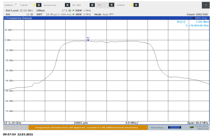
Figure 8.7-20: Conducted PSD on 802.11ac, Port B Low channel
