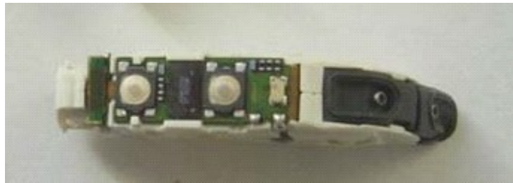
Radio module from the top side (button side)
