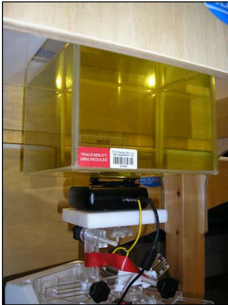
Figure 10. Positional photograph of the River ECG Cardiograph in normal user position, Belt Clip facing 0.0mm spacing from Phantom
