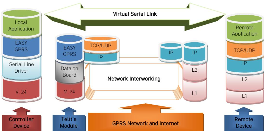
This particular implementation allows to the devices interfacing to the Telit GE865-QUAD module the use of the GPRS and Internet packet service without the need to have an internal TCP/IP stack since this function is embedded in the module.
