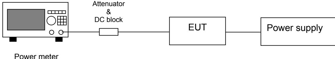
**Note 1:** The EUT was tested while in a continuous transmit mode and the worst case data rates are 1 Mbps for 802.11b and 6 Mbps for 802.11g. The EUT was tuned to a low, middle and high channel.
