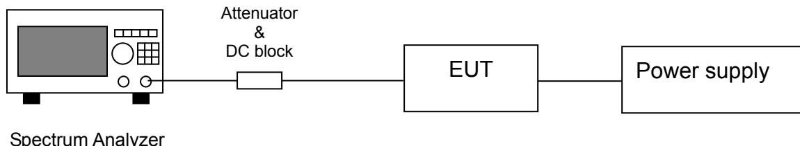
**Note:** The EUT was tested while in a continuous transmit mode and the worst case data rates are 1 Mbps for 802.11b and 6 Mbps for 802.11g. The EUT was tuned to a low, middle and high channel.
