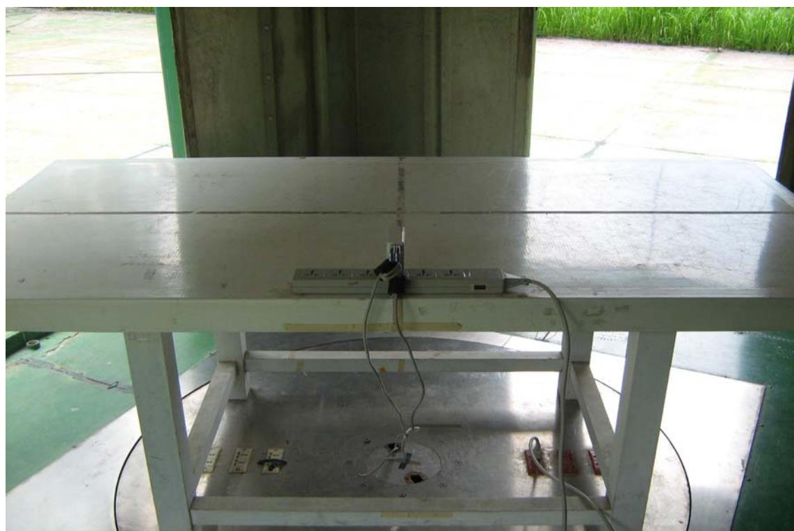
**RADIATED RF MEASUREMENT SETUP**
