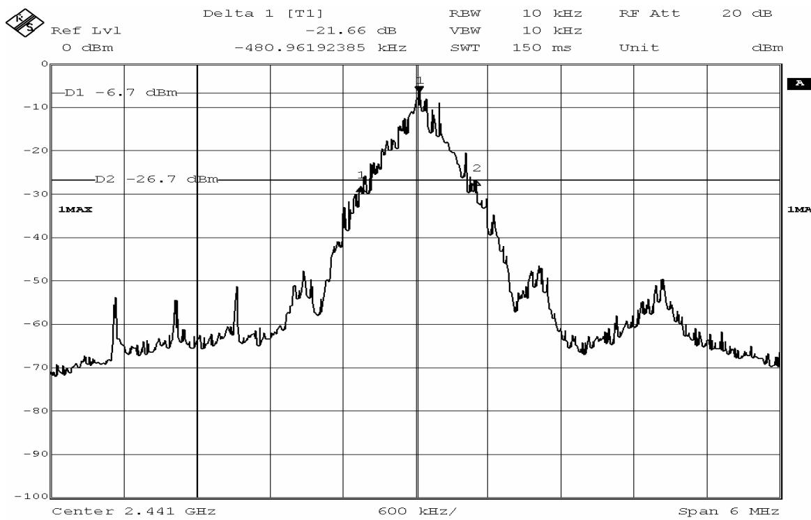
Remark: The 20dB Bandwidth = 'Delta 1' (468.9K) +'Delta 2' (468.9K) = 937.8 KHz
