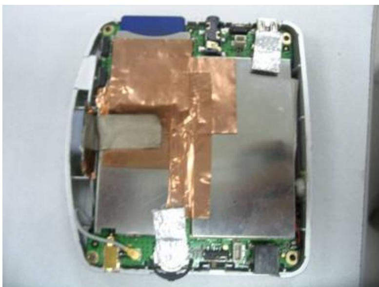
4. Add one filter for the DC-DC converter as the following figure shown.
