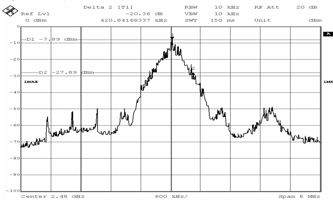
Remark: The 20dB Bandwidth = 'Delta 1' (456.9K) +'Delta 2' (420.8K) = 877.7 KHz
