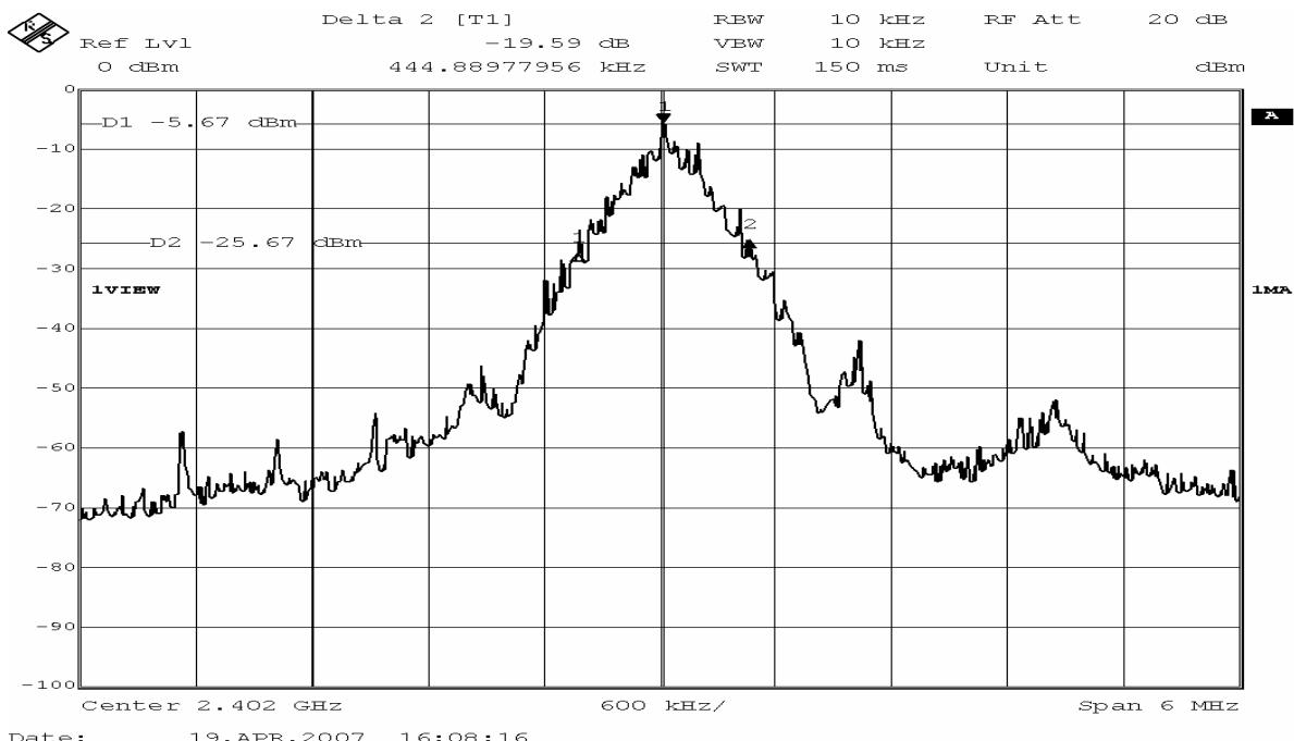
Remark: The 20dB Bandwidth = 'Delta 1' (444.9K) +'Delta 2' (444.9K) = 889.8 KHz
