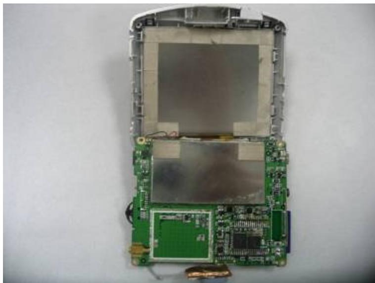
2. Add one electrolytic capacitor for the DC Input as the following figure shown.
