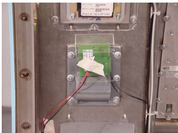
Photo 7: Set-up of the temperature sensor inside the system close to the detector antenna
