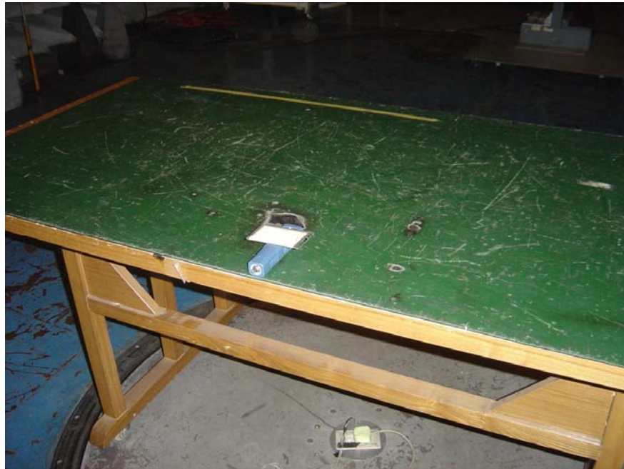
Maximized Radiated Emission Test Set-up- Reading Mode
