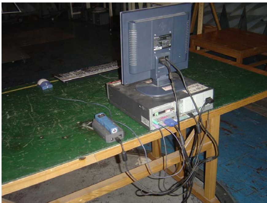
Maximized Radiated Emission Test Set-up - Communication Mode
