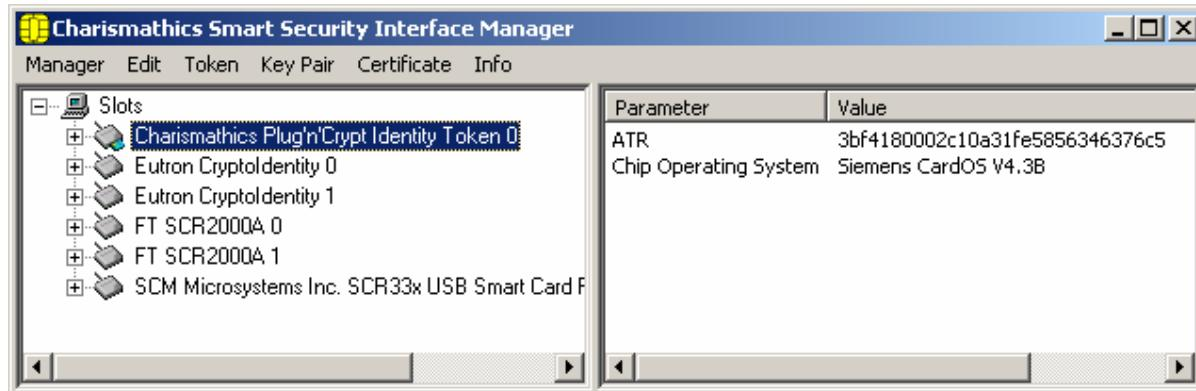
After you insert a smart card into the card reader, you can after one click on the smart card reader select the function "Open Token" with a click on the right mouse button. Alternatively you have the possibility to select this function under the menu "Manager".
