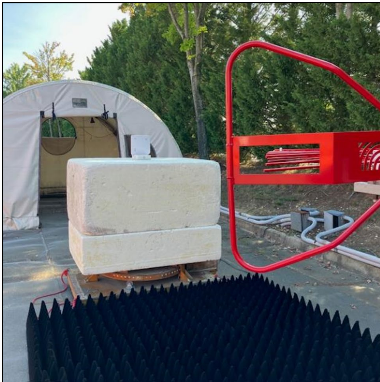
Photograph 3: Radiated Emissions, Above 1 GHz, Front
