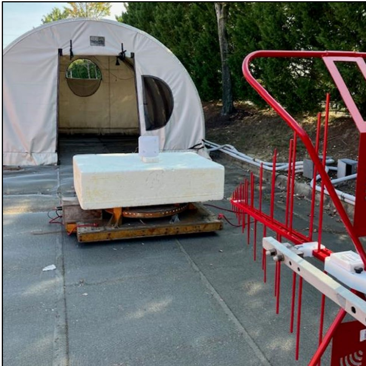
Photograph 1: Radiated Emissions, 30 MHz – 1 GHz, Front
