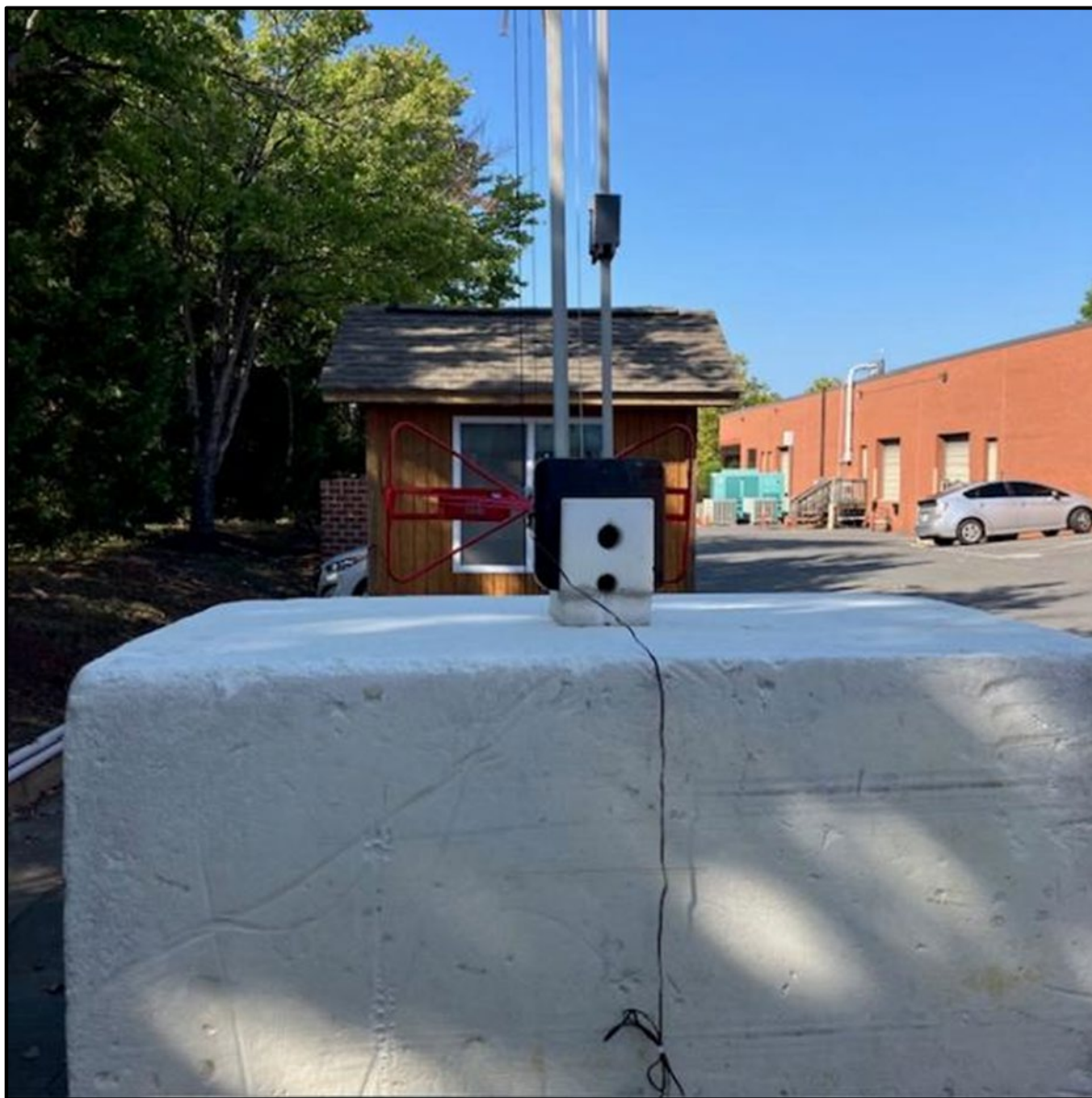
Photograph 4: Radiated Emissions, Above 1 GHz, Rear
