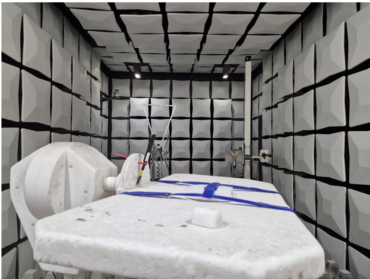
Photo 6: Test setup for radiated measurements, intentional radiator (fully anechoic chamber, above 1 GHz – 24 GHz;
