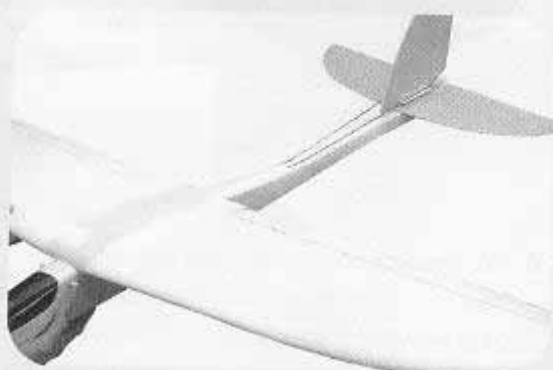
7. Lay the wings on the body of the plane and make the central line of the wings at the central line of the body.
