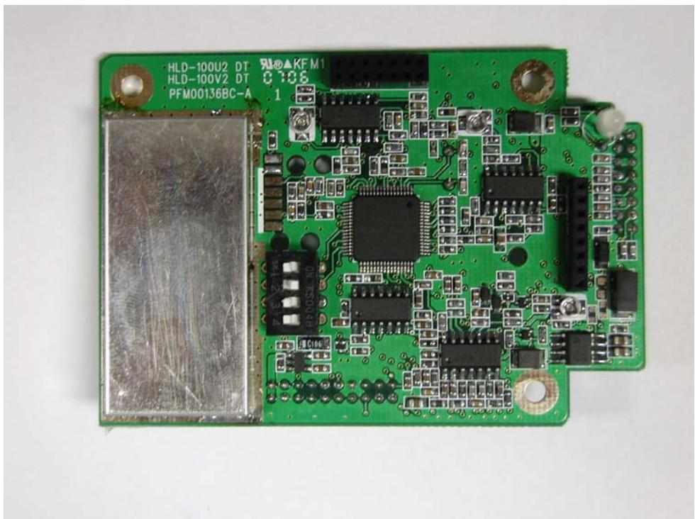
**Data PCB Side 1 with shield off - Front View**
