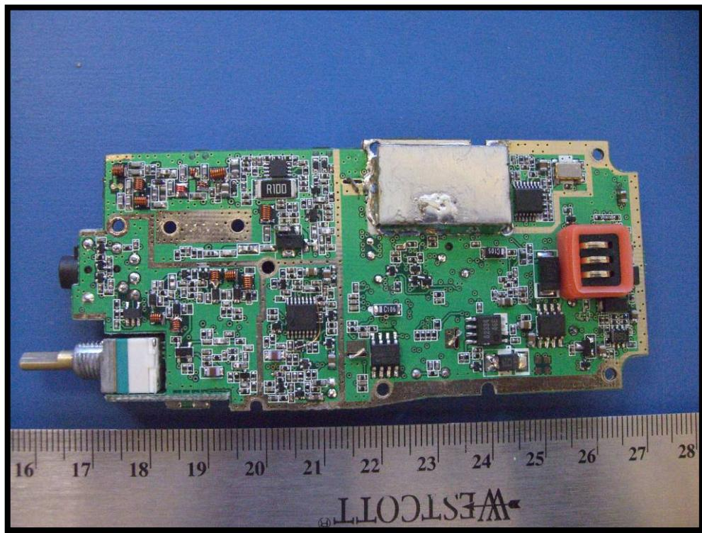
**EUT PCB Back View with Shield off**
