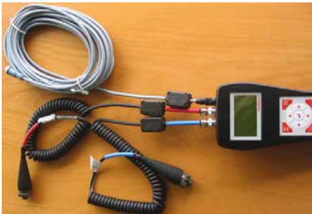
Ferrits fasten at the sensor cables
