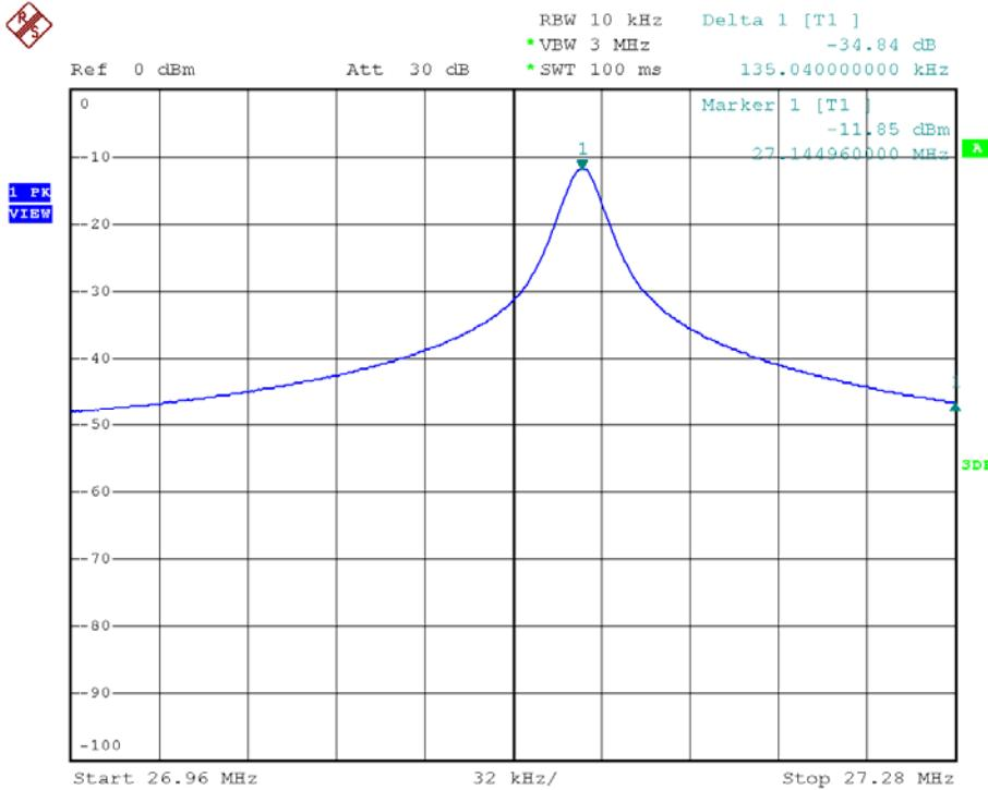
Bandedge Plot – Pursuant to FCC Part 15 Section 15. 227 Requirement (Pass)
