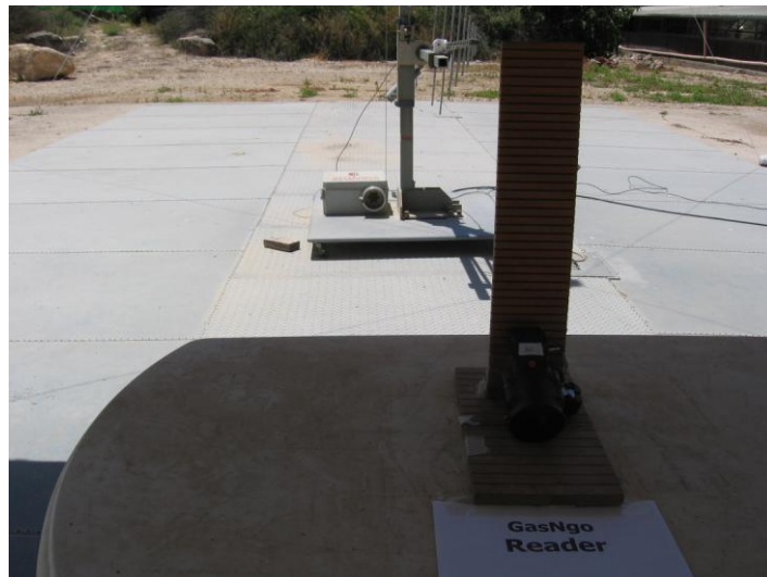
Figure 5. Radiated Emission Test
