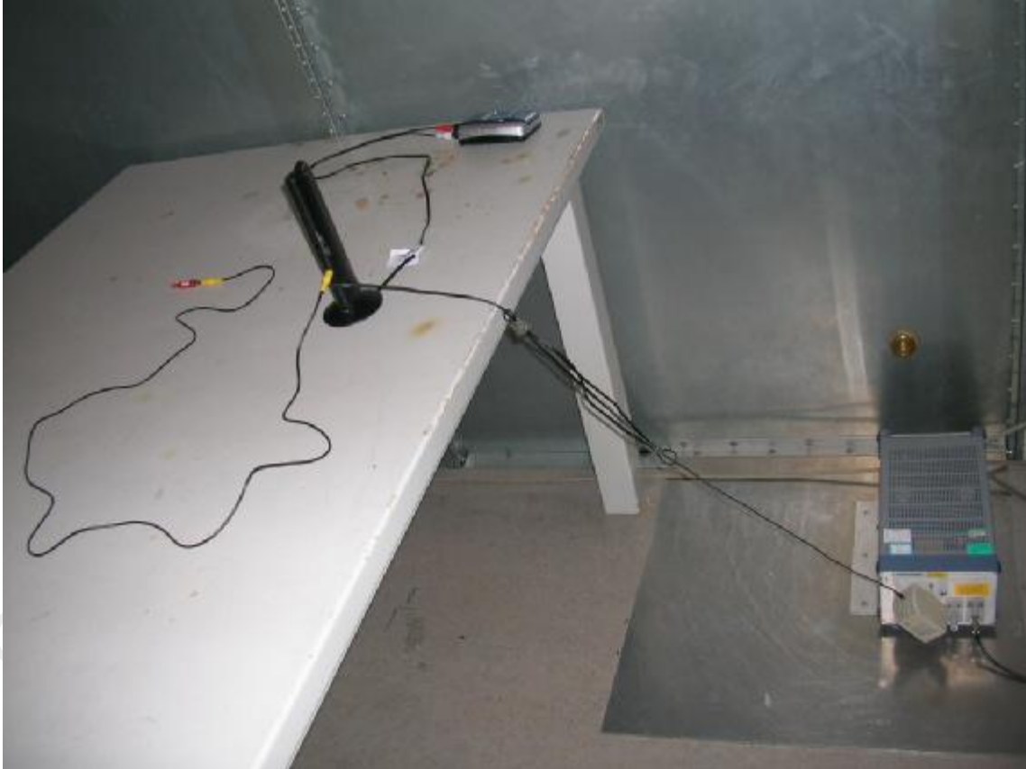
Measurement of Conducted Emission Test Set Up
