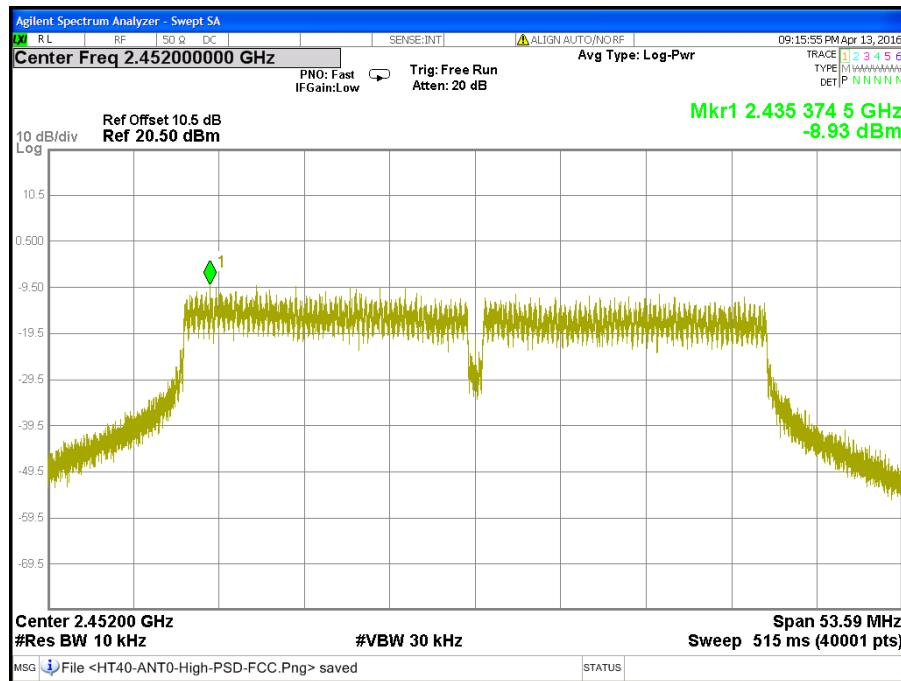
**CH Low (IEEE 802.11gn HT40 Mode / Chain 1)**
