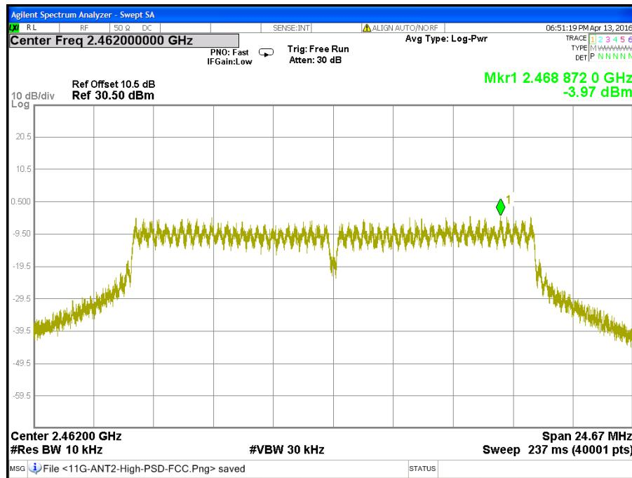
**CH Low (IEEE 802.11gn HT20 Mode / Chain 0)**
