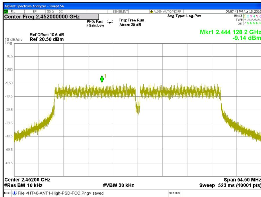
**CH Low (IEEE 802.11gn HT40 Mode / Chain 2)**
