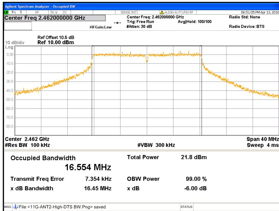
**CH Low (IEEE 802.11gn HT20 Mode / Chain 0)**
