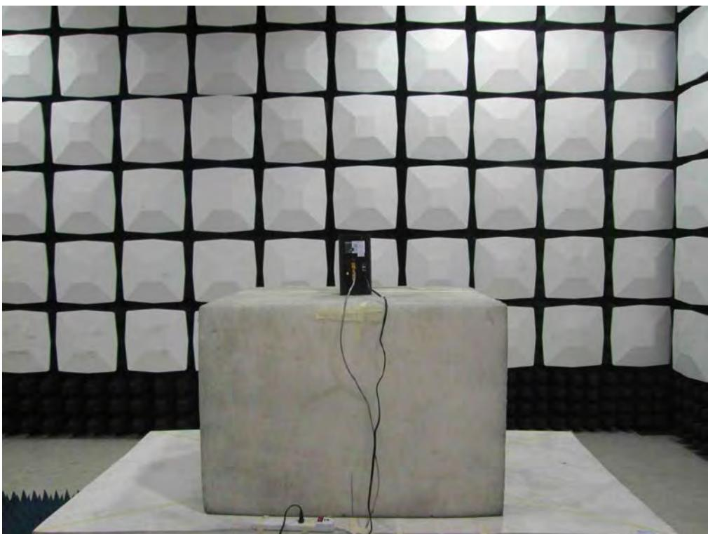
**ANTENNA PORT CONDUCTED RF MEASUREMENT SETUP**
