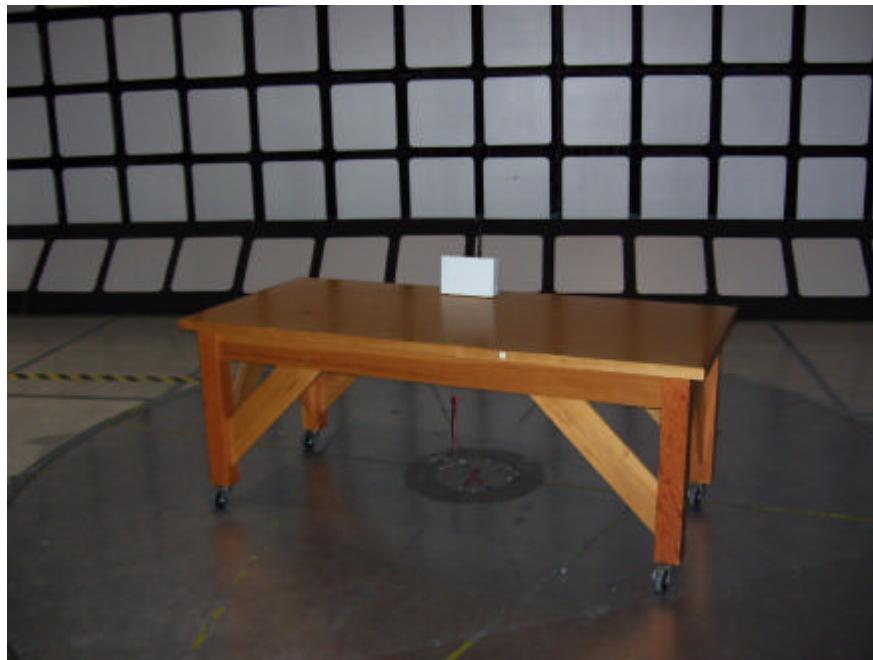
Figure 14 - Radiated Emissions Test Setup, Dipole Antenna
