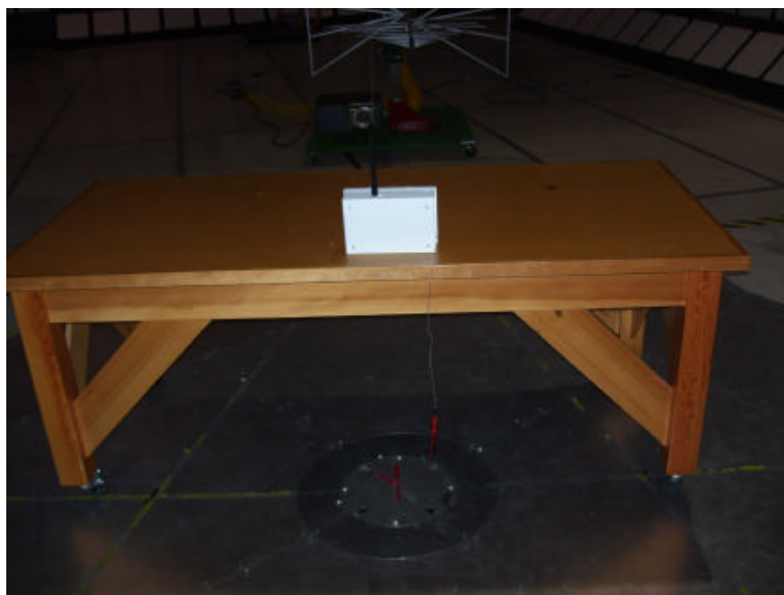
Figure 15 - Radiated Emissions Test Setup, Dipole Antenna
