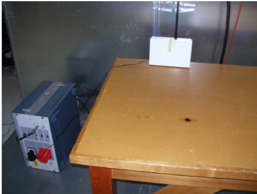
Figure 18 - Conducted Emissions Test Setup
