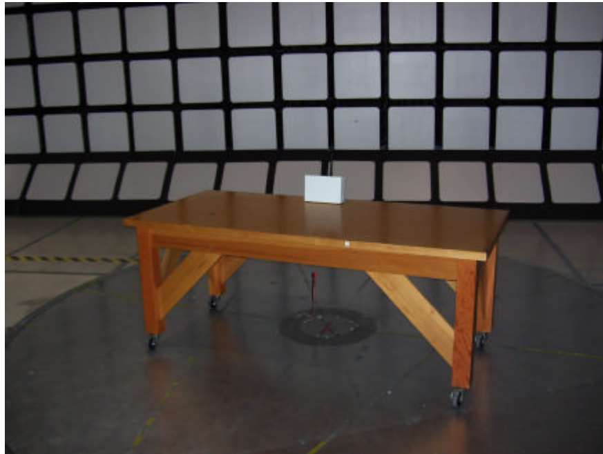
Figure 14 - Radiated Emissions Test Setup, Dipole Antenna
