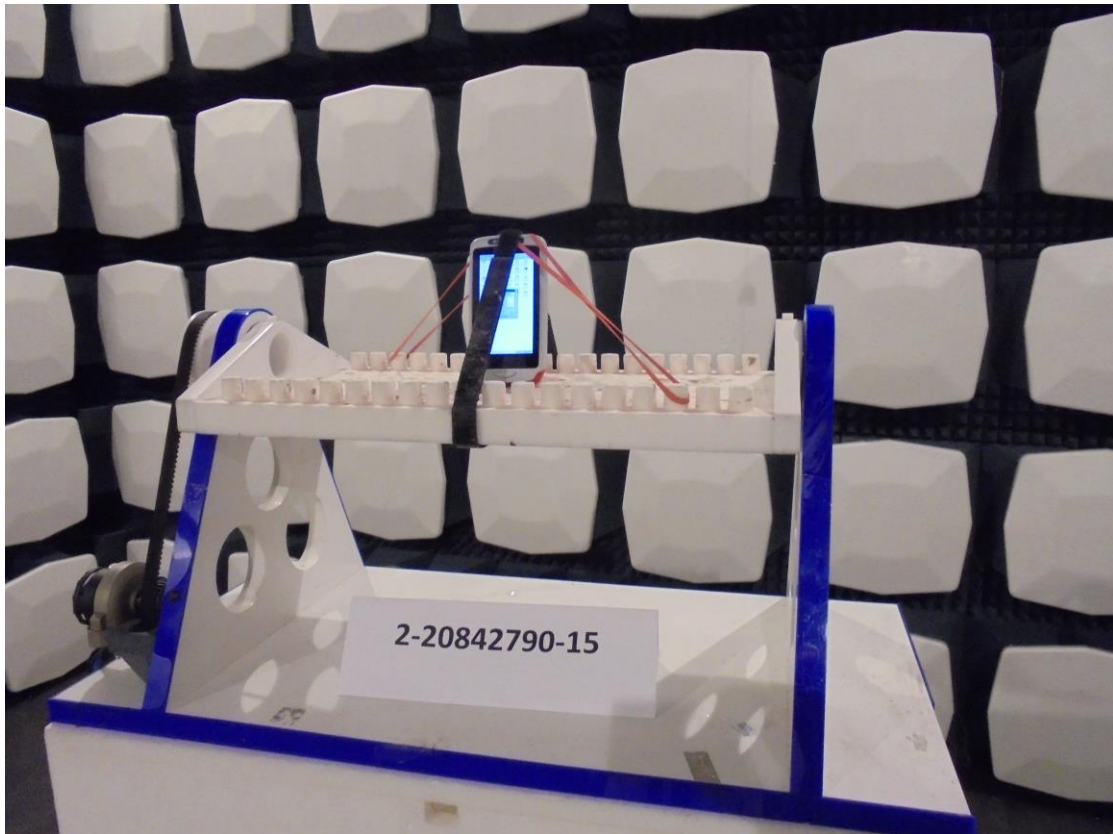
Photograph 18: Radiated measurement set-up (close up view_front side) _EUT 0°
