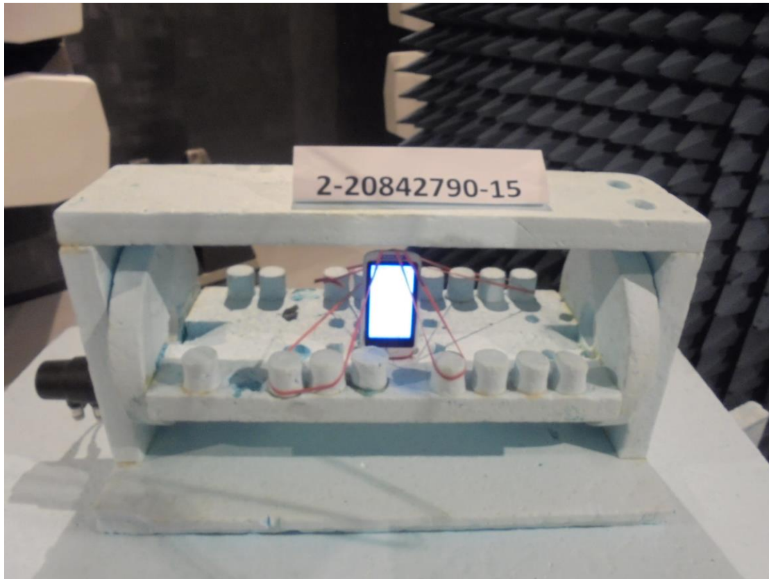
Photograph 10: Radiated measurement set-up (close up view_front side)_EUT 0°
