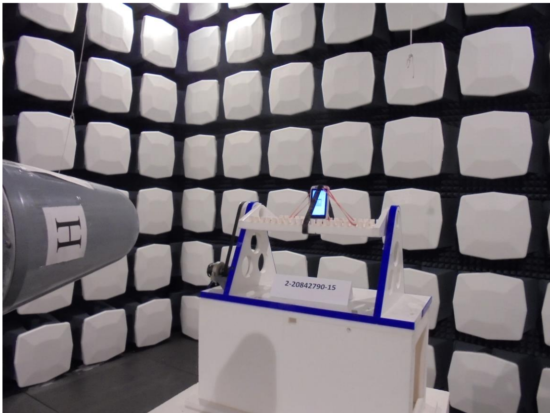
Photograph 16: Radiated measurement set-up (overview_front side) _EUT 0°
