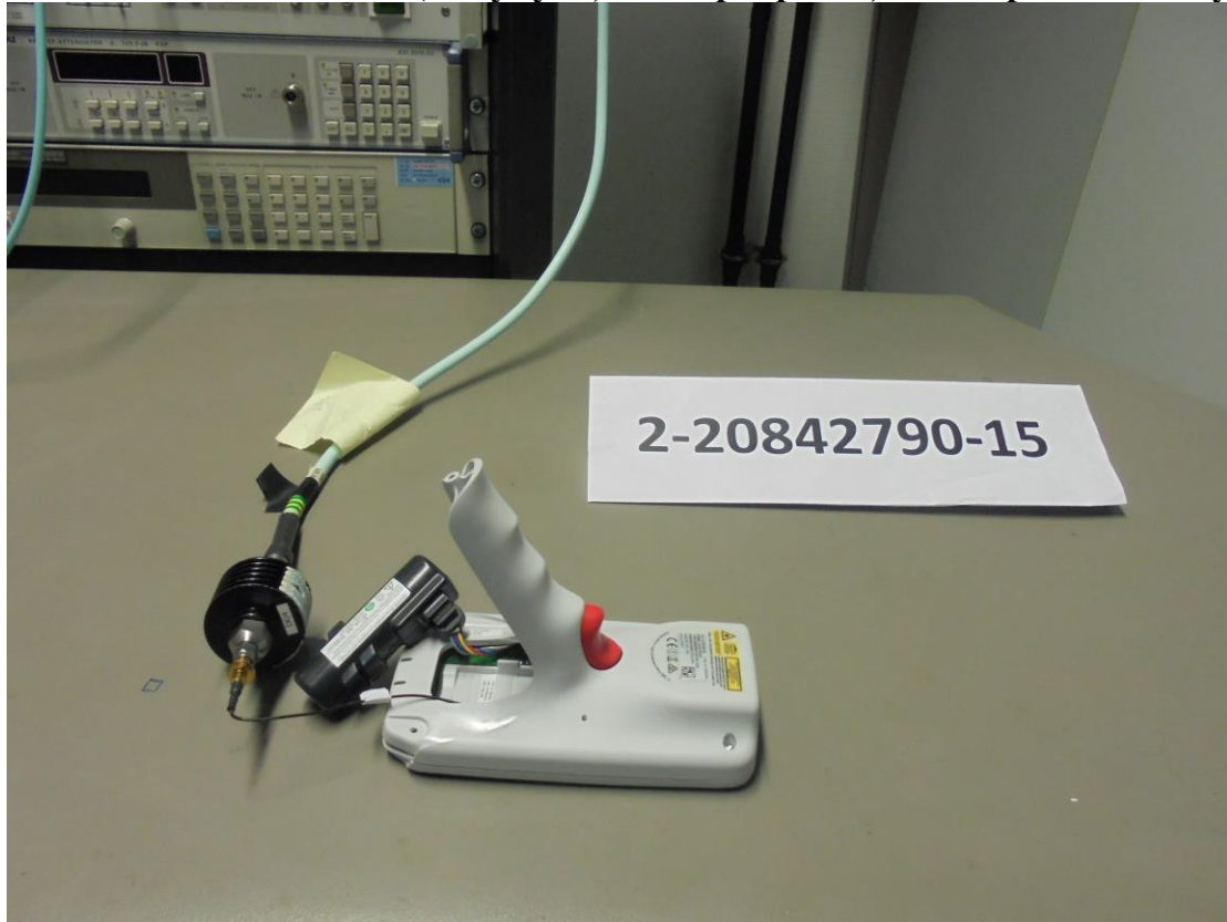
Photograph 1: Conducted measurement set-up (close up view_front side)
