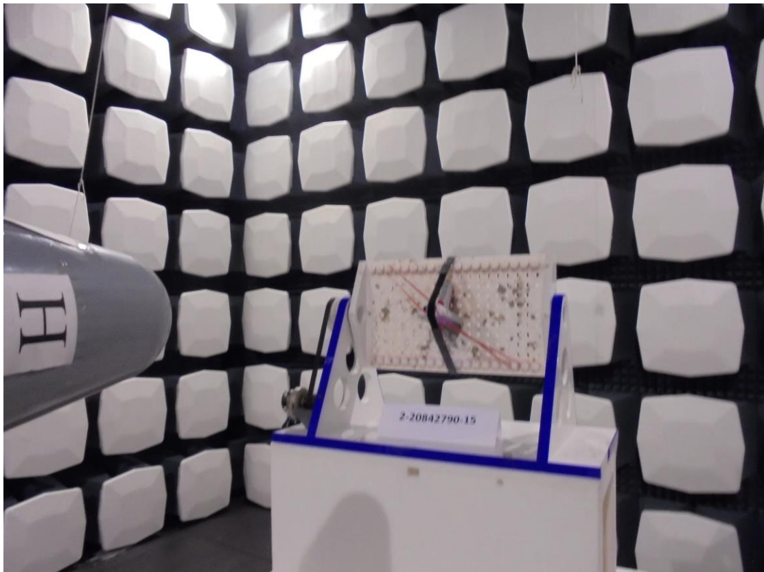
Photograph 17: Radiated measurement set-up (overview_front side) _EUT 90°
