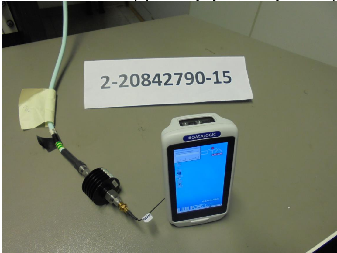
Photograph 1: Conducted measurement set-up (close up view_front side)
