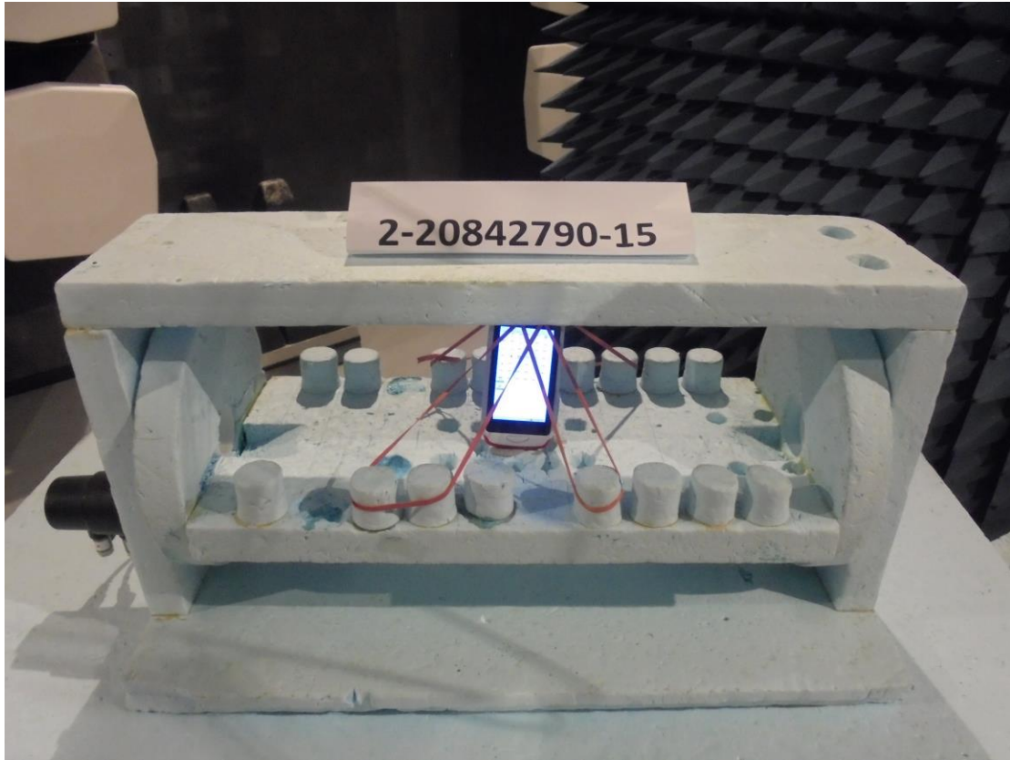
Photograph 10: Radiated measurement set-up (close up view_front side)_EUT 0°
