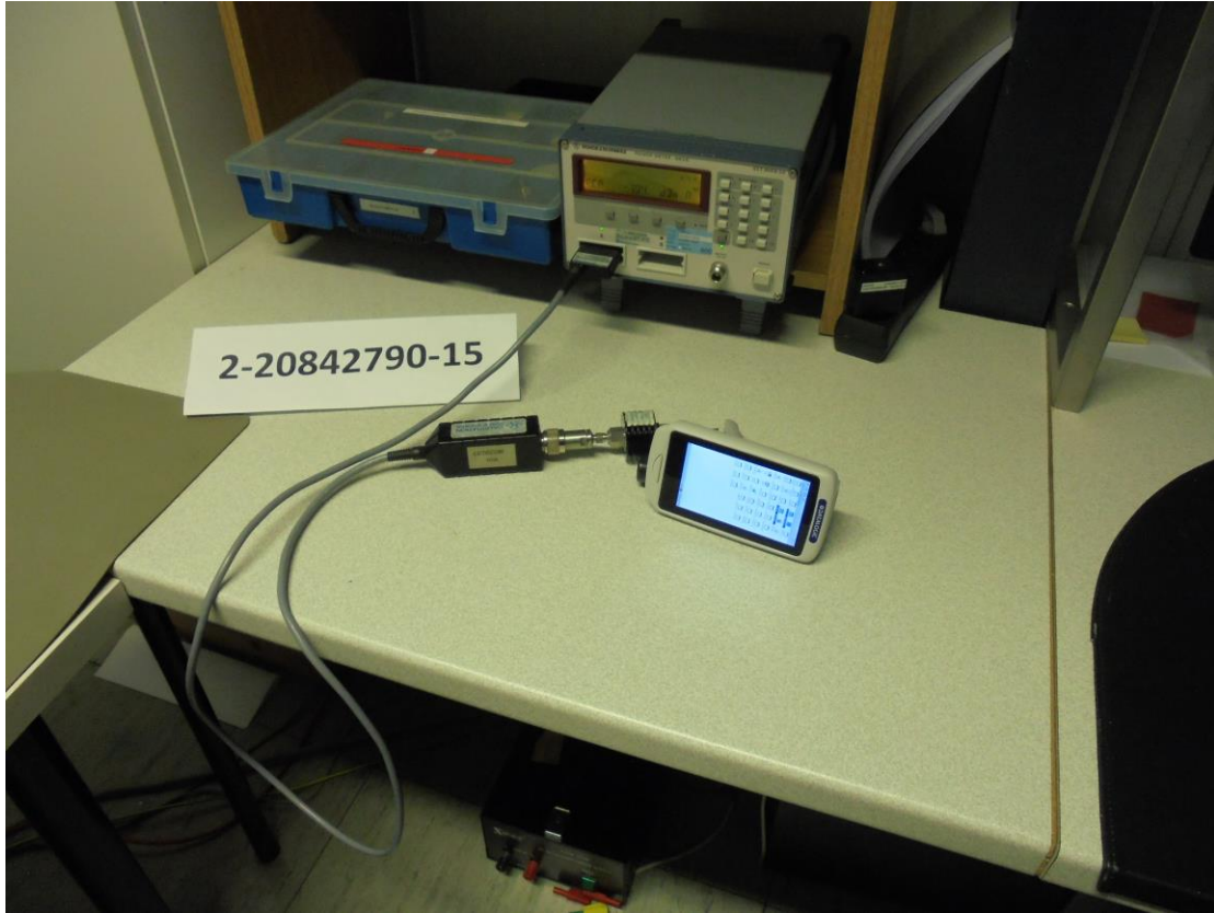
Photograph 3: Conducted measurement power meter set-up (overview_front side)
