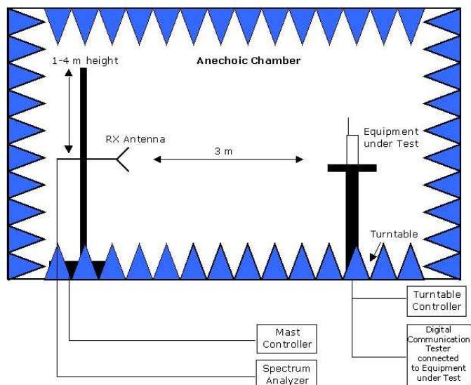
Setup in the Anechoic chamber. For measurements below 1 GHz the ground was replaced by a conducting ground plane.
