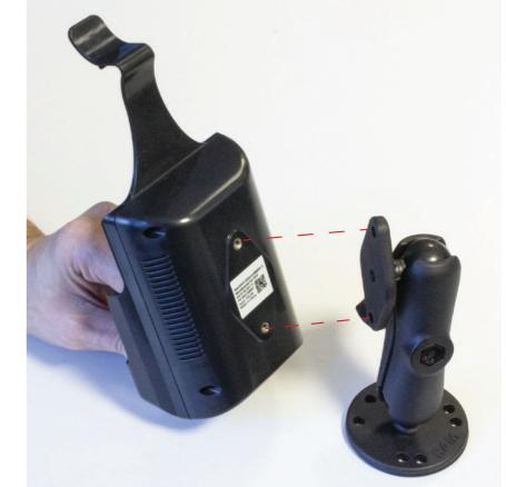
2. Secure the adjustable arm to the rear of the dock using two screws M5X10 and two nuts M5:
