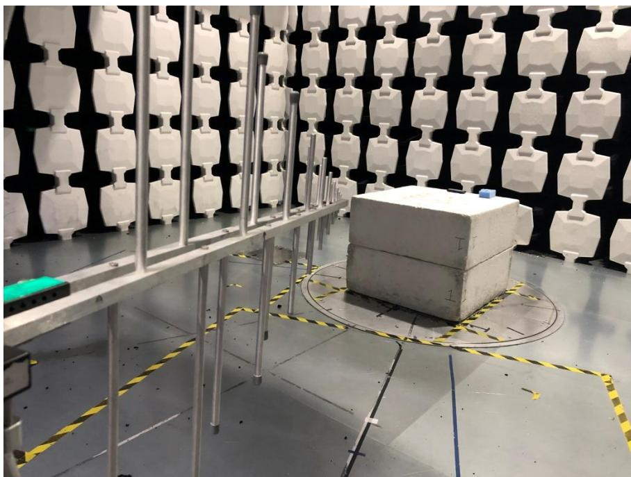
Description: Radiated Emission Test Setup
