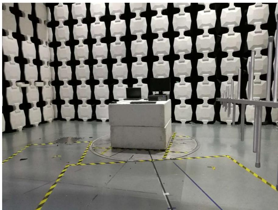
Description: Radiated Emission Test Setup
