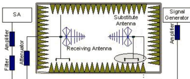
In the chamber, an substitution antenna for the frequency band of interest is placed at the reference point
