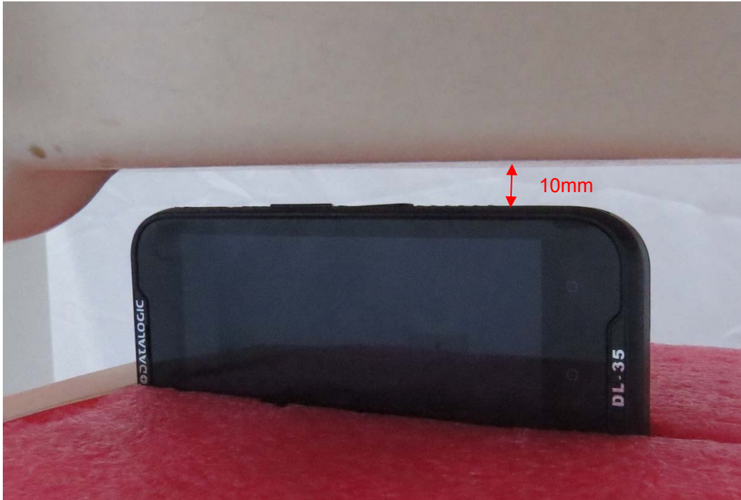
Picture 14: Right Side, the distance from handset to the bottom of the Phantom is 10mm
