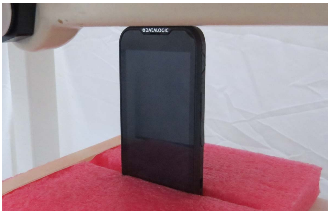
Picture 17: Top Side, the distance from handset to the bottom of the Phantom is 0mm
