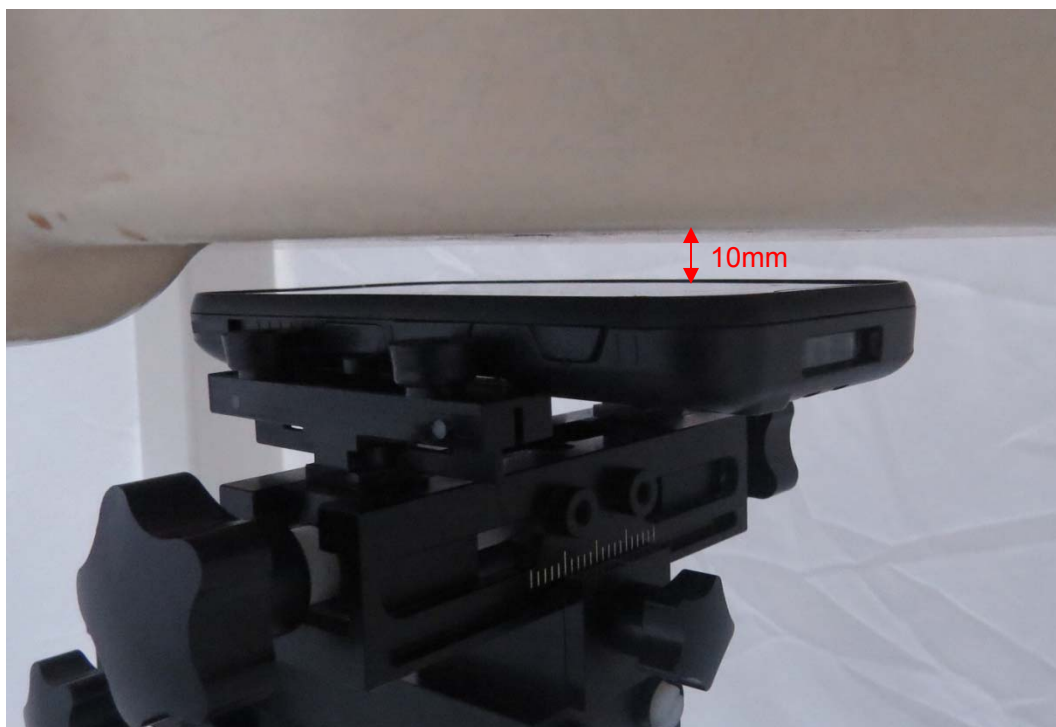
Picture 12: Front Side, the distance from handset to the bottom of the Phantom is 10mm
