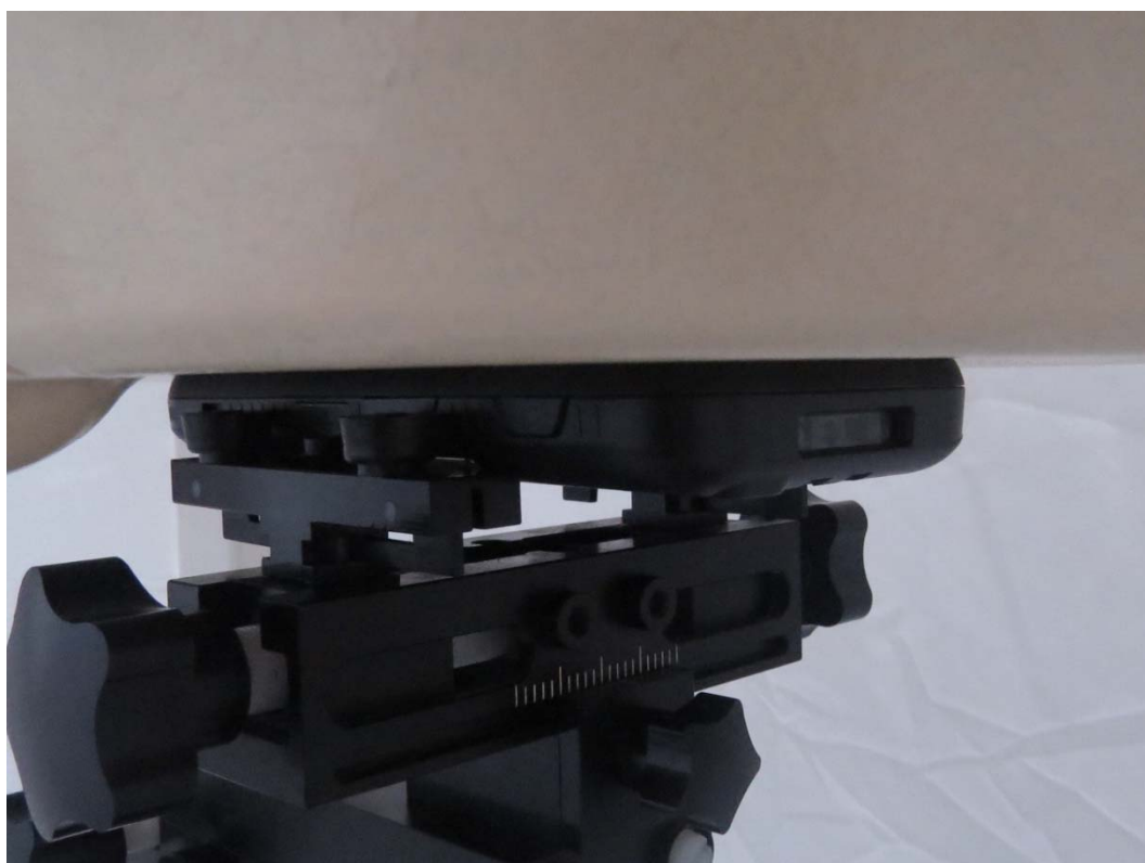
Picture 13: Front Side, the distance from handset to the bottom of the Phantom is 0mm
