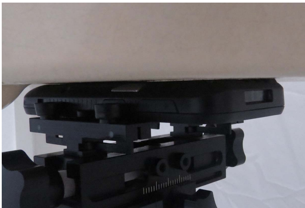
Picture 11: Back Side, the distance from handset to the bottom of the Phantom is 0mm
