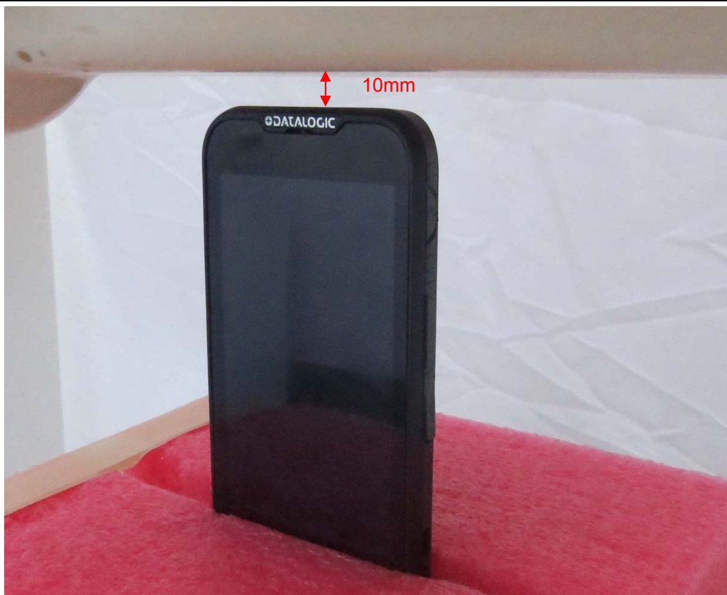
Picture 16: Top Side, the distance from handset to the bottom of the Phantom is 10mm
