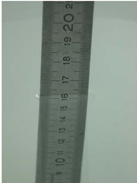
Fig. 13: Liquid depth for 2450 MHz body worn measurements.
