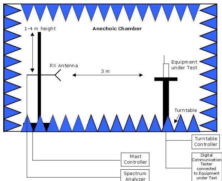
**Drawing 1:** Setup in the Anechoic chamber:
